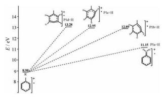
FIG. 2 The dissociation channels for toluene cation to produce fragment ions,  ${\rm C_7H_7}^+({\rm P1})$  calculated at the G3B3 level. The energy of neutral toluene is defined to be zero.
