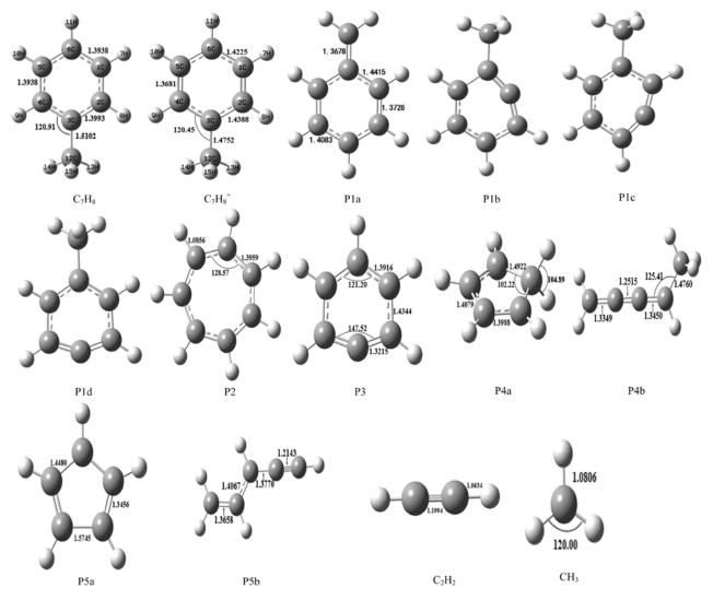
FIG. 7 The geometries of the neutral toluene, its cation and its fragments (ions and neutrals) at the B3LYP/6-311++G(d,p) level. Bond length is in unit of Å and bond angel in unit of ( $^{\circ}$ ).
