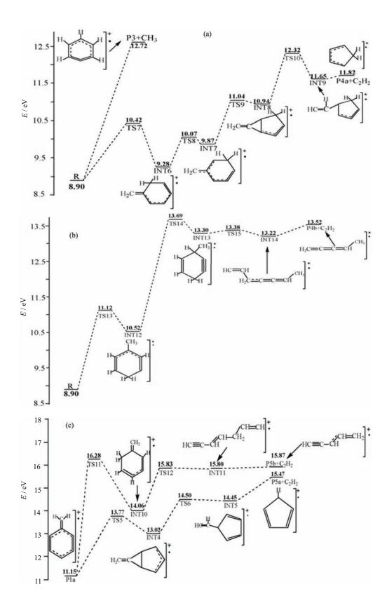
FIG. 4 The dissociation channels for toluene cation to produce fragment ions  $C_6H_5^+(P3)$  and  $C_5H_6^+(P4a)$ ,  $C_5H_6^+(P4b)$  and  $C_5H_5^+$ , calculated at the G3B3 level. The energy of neutral toluene is defined to be zero.
