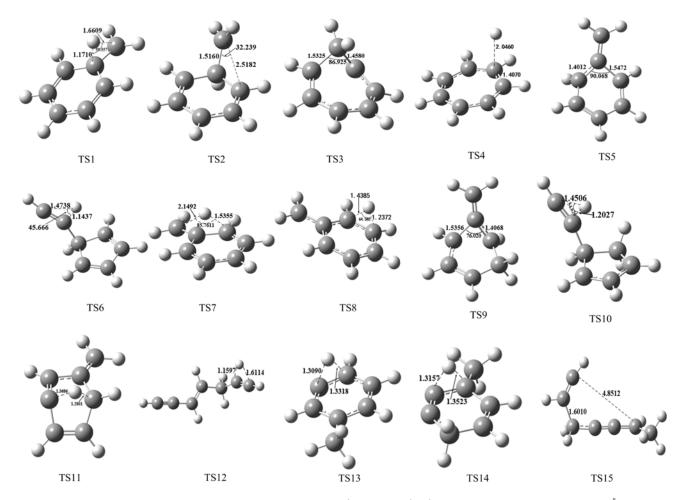
FIG. 5 The geometries of the transition states at the B3LYP/6-311++G(d,p) level. Bond length is in unit of Å and bond angel in unit of ( $^{\circ}$ ).
