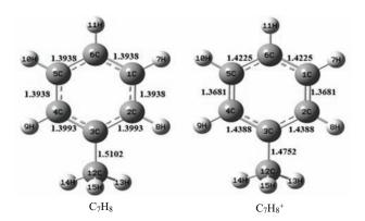
FIG. 1 The optimized geometries of the neutral toluene and its cation. (a)  $C_7H_8$ , (b)  $C_7H_8^+$ . Bond length is in unit of Å.
