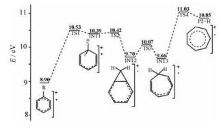
FIG. 3 The dissociation channel for toluene cation to produce fragment ion,  $\mathrm{C_7H_7}^+(\mathrm{P2})$  calculated at the G3B3 level. The energy of neutral toluene is defined to be zero.
