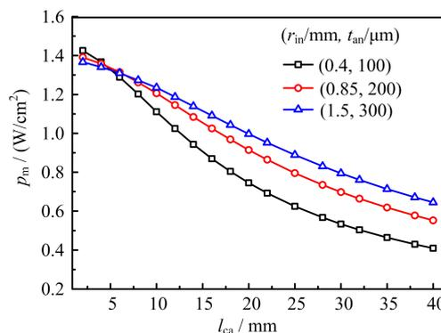
FIG. 4  $p_m$  by double-terminal anode current collection (DTACC) vs.  $l_{ca}$  for  $(r_{in}, t_{an})=(0.4$  mm,  $100 \mu m)$ ,  $(0.85$  mm,  $200 \mu m)$  and  $(1.5$  mm,  $300 \mu m)$ .
