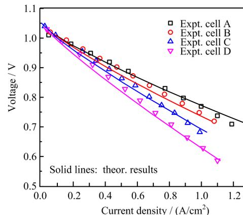
FIG. 2 Comparison of the theoretical and experimental  $I$ - $V$  curves of four single cells A, B, C, D that differ in the distance  $d$  between the cathode and the anode current collector with  $d=2, 5, 8, 14$  cm, respectively.
