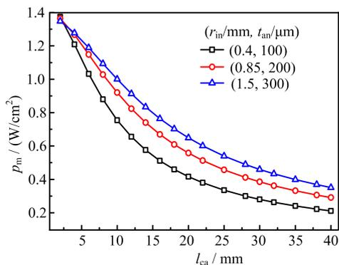
FIG. 3 The maximum area specific power density,  $p_m$ , by single-terminal anode current collection (STACC) vs. the cathode length,  $l_{ca}$ , for  $(r_{in}, t_{an})=(0.4$  mm,  $100 \mu m)$ ,  $(0.85$  mm,  $200 \mu m)$  and  $(1.5$  mm,  $300 \mu m)$ .
