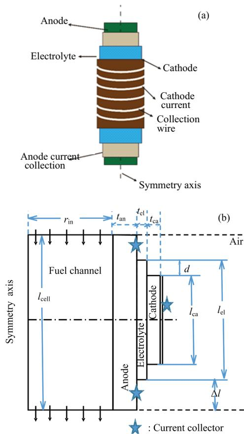
FIG. 1 Schematic diagram of mtSOFC. (a) 3D structure, (b) 2D computational domain.
