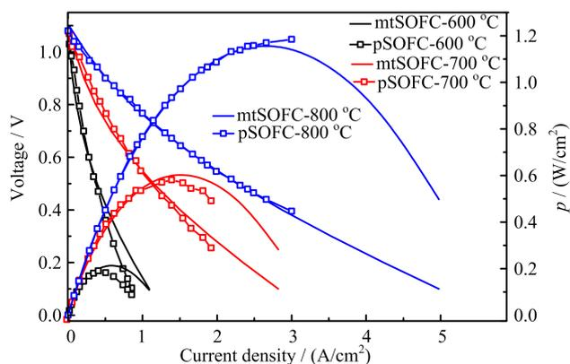
FIG. 5 Comparison of  $I$ - $V$  and  $I$ - $p$  relations of mtSOFC and pSOFC ( $p$ : area specific power density).
