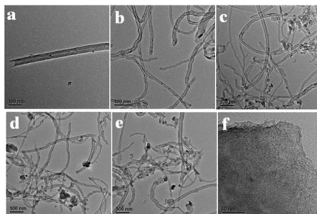
FIG. 2 TEM patterns of the (a) pure CNTs, K-Co-Mo/CNTs with different Mo loading of (b) 10 wt%, (c) 30 wt%, (d) 40 wt%, (e) 50 wt%; and (f) K-Co-Mo/AC with Mo loading of 30 wt%.
