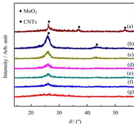
FIG. 1 XRD patterns of (a) unsupported K-Co-Mo, (b) pure CNTs, K-Co-Mo/CNTs with different Mo loading of (c) 10 wt%, (d) 30 wt%, (e) 40 wt%, (f) 50 wt%, and (g) K-Co-Mo/AC with Mo loading of 30 wt%.
