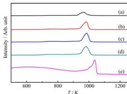
FIG. 4  $H_2$ -TPD of the K-Co-Mo/CNTs with different Mo loading of (a) 10 wt%, (b) 30 wt%, (c) 40 wt%, (d) 50 wt% and (e) K-Co-Mo/AC with Mo loading of 30 wt%.
