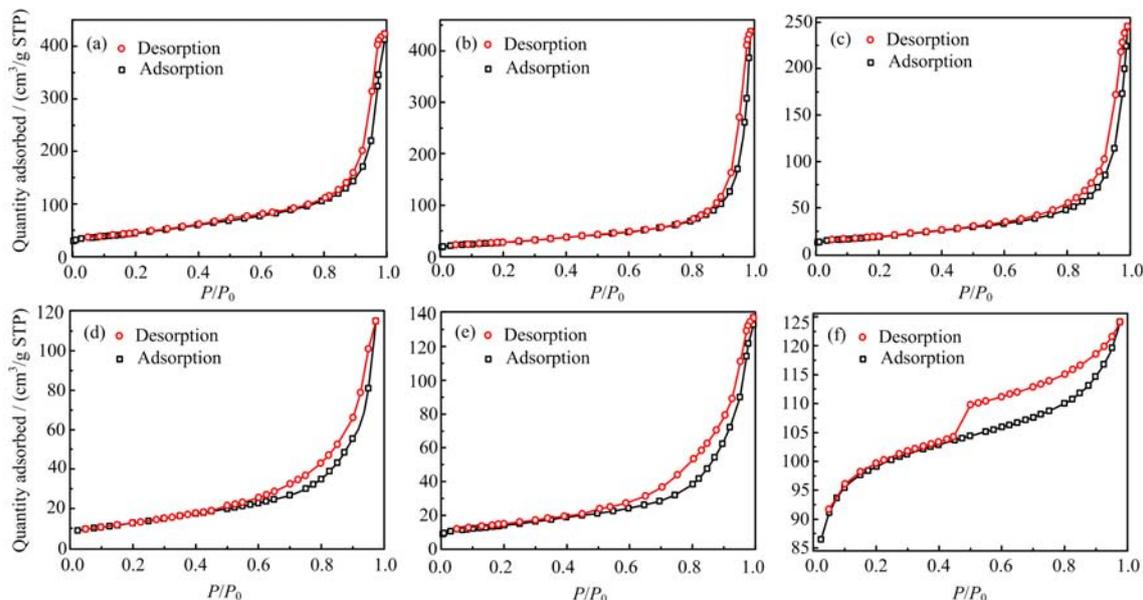
FIG. 3 Nitrogen adsorption-desorption isotherms of (a) pure CNTs, K-Co-Mo/CNTs with different Mo loading of (b) 10 wt%, (c) 30 wt%, (d) 40 wt%, (e) 50 wt%, and (f) K-Co-Mo/AC with Mo loading of 30 wt%.
