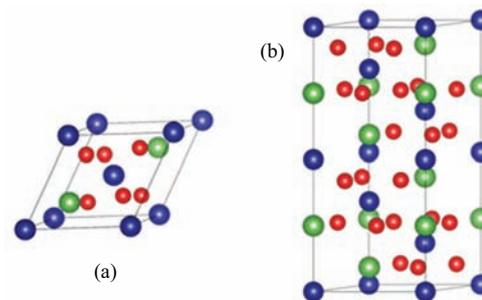
FIG. 1 (a) Rhombohedral primitive cell and (b) hexagonal unit cells of  $\text{LaCoO}_3$ . Green, blue, and red balls represent La, Co and O atoms, respectively.
