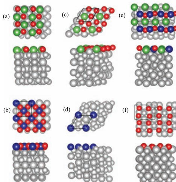
FIG. 2 The top and side views of optimized (a)  $(\bar{1}\bar{1}02)$ - $\text{LaO}$ , (b)  $(\bar{1}\bar{1}02)$ - $\text{CoO}_2$ , (c)  $(0001)$ - $\text{LaO}_3$ , (d)  $(0001)$ - $\text{Co}$ , (e)  $(\bar{1}\bar{1}04)$ - $\text{LaCoO}$ , and (f)  $(\bar{1}\bar{1}04)$ - $\text{O}_2$ . Green, blue, and red balls represent La, Co, and O atoms, respectively.
