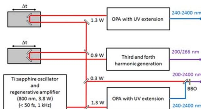
FIG. 2 Schematic overview of the femtosecond laser system.
