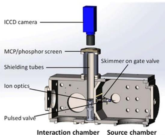
FIG. 1 Schematic view of the velocity map imaging spectrometer.
