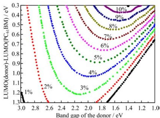
FIG. 3 Predicted PCE for BTBPD-PC<sub>61</sub>BM cell with the Scharber diagram.
