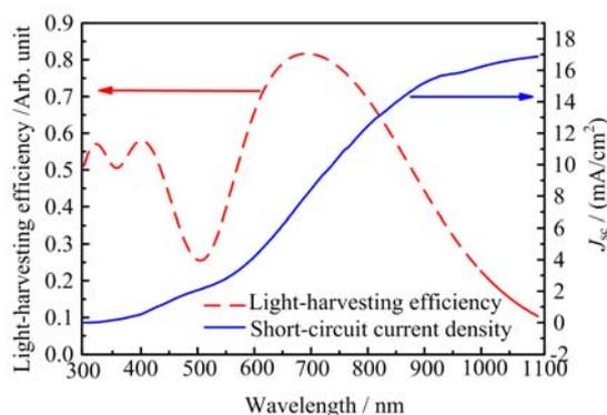
FIG. 5 Predicted  $J_{sc}$  and  $\eta_{\lambda}$  for BTBPD-PC<sub>61</sub>BM cell.
