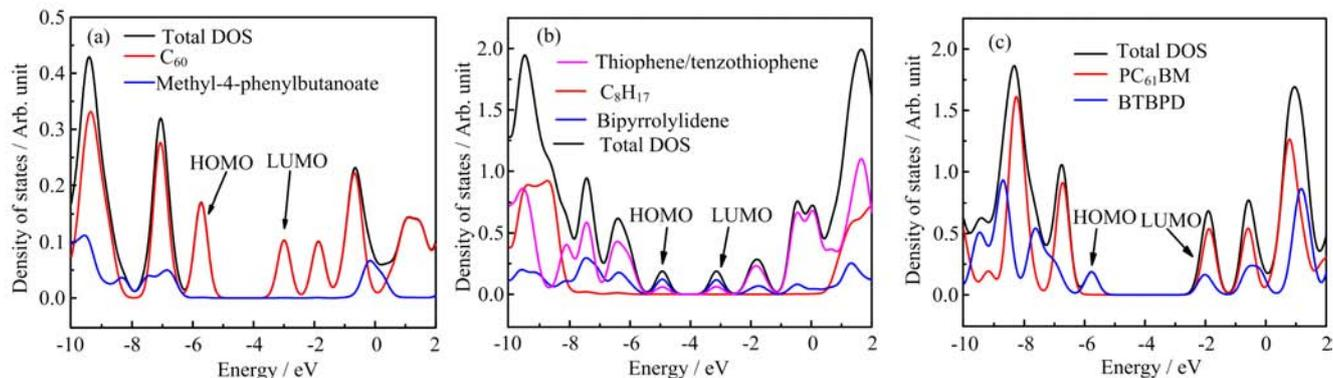
FIG. 2 Total density of states and partial density of states of (a) PC<sub>61</sub>BM, (b) BTBPD, and (c) PC<sub>61</sub>BM-BTBPD complex.
