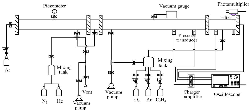
FIG. 1 Schematic diagram of shock tube apparatus.
