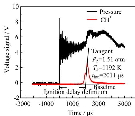
FIG. 2 Definition of ignition delay time.  $P_5=1.51$  atm,  $T_5=1192$  K,  $\tau_{\text{ign}}=2011$   $\mu\text{s}$ .
