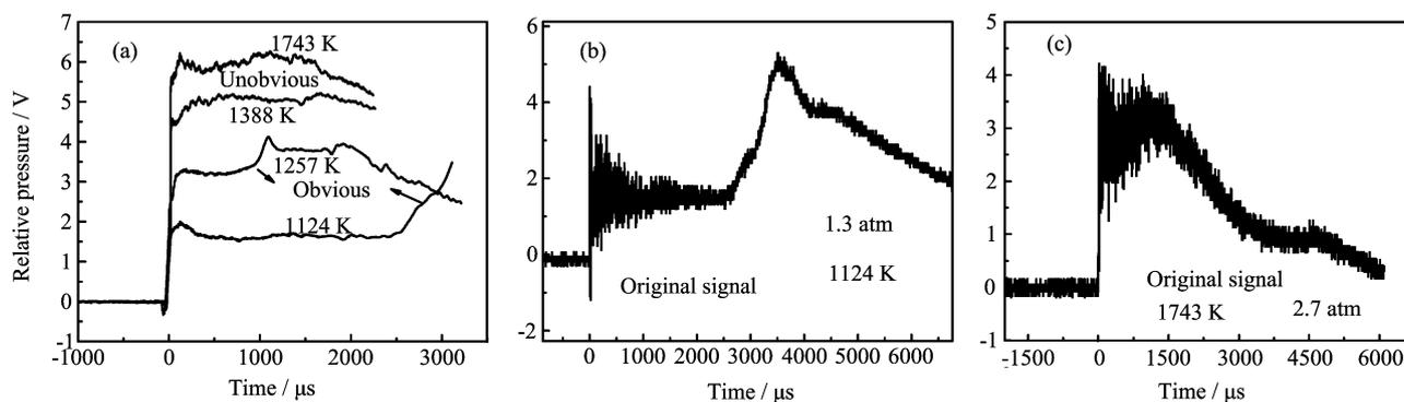
FIG. 3 (a) Pressure response of mild ignition (filtered with second order Savitzky-Golay polynomial, 96% Ar), (b) a low temperature case (1124 K), (c) a high temperature case (1743 K).
