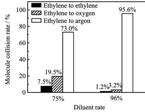
FIG. 7 Single ethylene molecule collision rate in 75% and 96% Ar diluents conditions.
