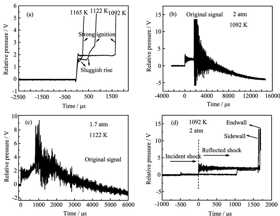
FIG. 4 (a) Pressure response of strong ignition, filtered with second order Savitzky-Golay polynomial, 75% Ar, (b) direct strong ignition, (c) deflagration to detonation transition (DDT), (d) pressure traces of remote ignition.
