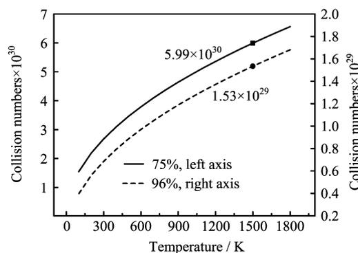
FIG. 8 Collision numbers under different temperature regions (ethylene to oxygen, 96% vs. 75% Ar diluent conditions).
