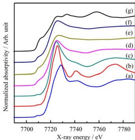
FIG. 3 Co K-edge XANES spectra of (a) standard  $\text{Co}_3\text{O}_4$ , (b) standard  $\text{CoO}$ , (c) fresh K-Co-Mo/AC catalyst, (d)  $\text{H}_2$ -reduced catalyst, (e) syngas-reduced catalyst, (f) CO-reduced catalyst, and (g) Co foil.
