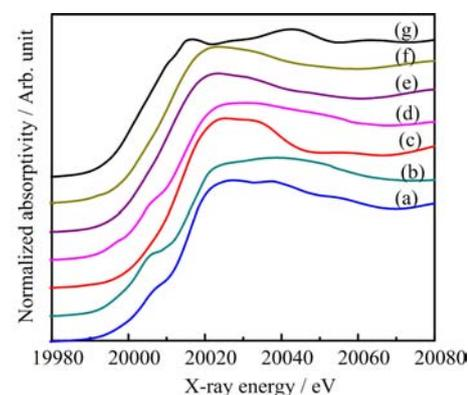
FIG. 2 Mo K-edge XANES spectra of (a) standard MoO<sub>3</sub>, (b) fresh K-Co-Mo/AC catalyst, (c) standard MoO<sub>2</sub>, (d) CO-reduced catalyst, (e) H<sub>2</sub>-reduced catalyst, (f) syngas-reduced catalyst, and (g) Mo foil.
