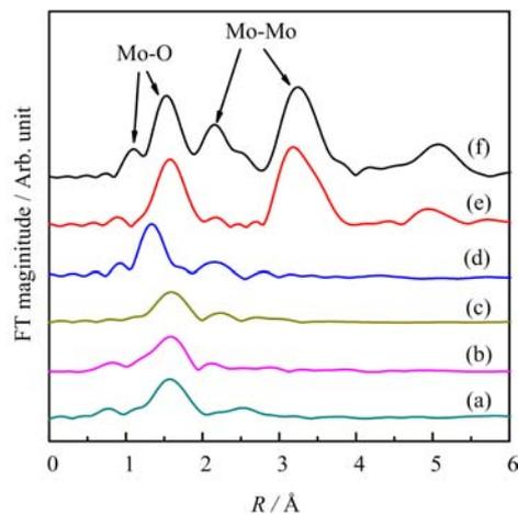
FIG. 4 Fourier transforms of Mo K-edge EXAFS of (a)  $\text{H}_2$ -reduced catalyst, (b) syngas-reduced catalyst, (c) CO-reduced catalyst, (d) fresh K-Co-Mo/AC catalyst, (e) standard  $\text{MoO}_3$ , and (f) standard  $\text{MoO}_2$ .
