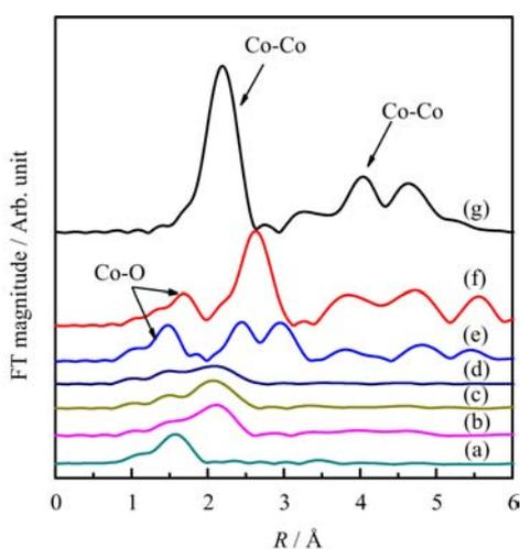
FIG. 5 Fourier transforms of Co K-edge EXAFS of (a) fresh K-Co-Mo/AC catalyst, (b)  $H_2$ -reduced catalyst, (c) syngas-reduced catalyst, (d) CO-reduced catalyst, (e) standard  $Co_3O_4$ , (f) standard CoO, and (g) Co foil.
