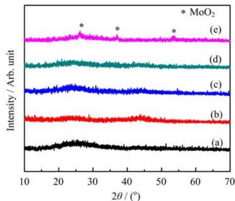
FIG. 1 XRD patterns of (a) fresh supported K-Co-Mo/AC catalyst, (b) H<sub>2</sub>-reduced catalyst, (c) syngas-reduced catalyst, (d) CO-reduced catalyst, and (e) fresh unsupported K-Co-Mo catalyst.
