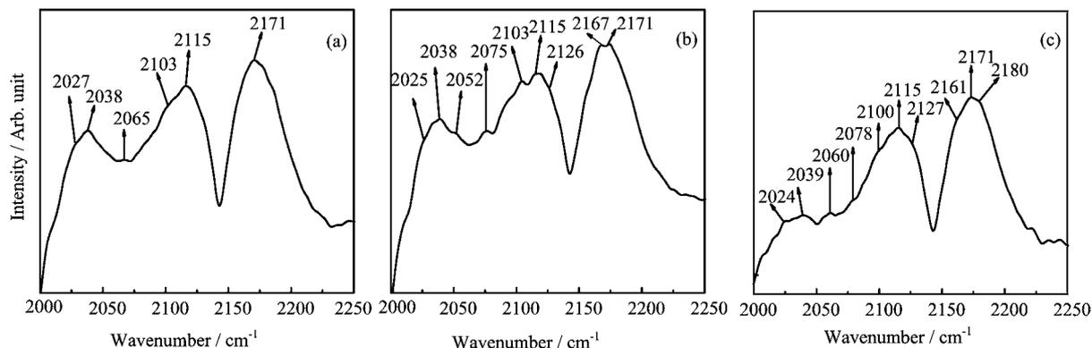
FIG. 6 *In situ* DRIFTS of CO adsorption on (a)  $H_2$ -reduced catalyst, (b) syngas-reduced catalyst, and (c) CO-reduced catalyst.
