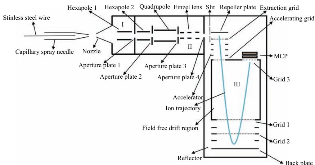
FIG. 1 Schematic diagram of the experiment setup containing a nano-electrospray ionization source, an ion transmission and focus system and a reflectron time-of-flight mass spectrometer.
