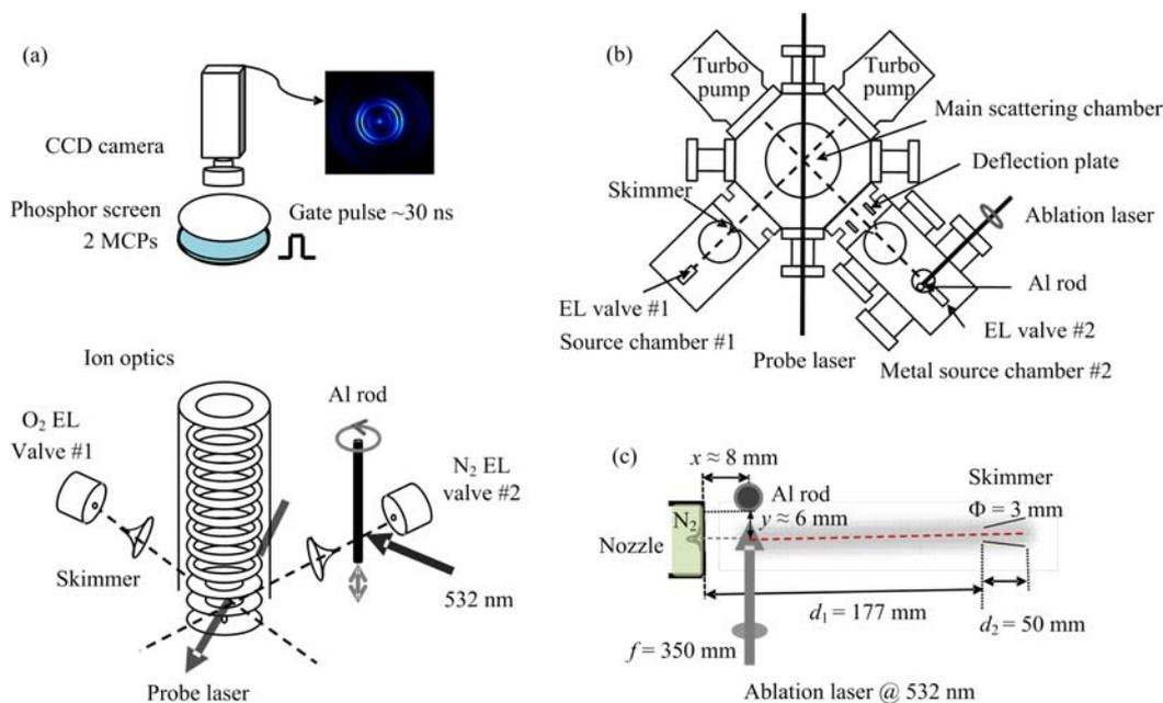
FIG. 1 Schematic view of (a) crossed-beam apparatus for studying metal atomic reaction dynamics, (b) crossed-beam chambers, and (c) supersonic aluminium atomic beam source generated by laser ablation.
