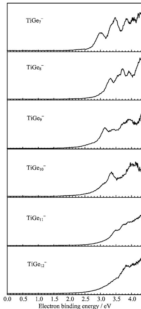
FIG. 1 Photoelectron spectra of  $\text{TiGe}_n^-$  ( $n=7-12$ ) clusters recorded with 266 nm photons.
