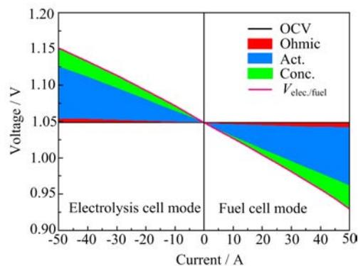
FIG. 5 Voltage of RSOC system versus current at 1 atm,  $950\text{ }^\circ\text{C}$  and with the state of charge 95%.
