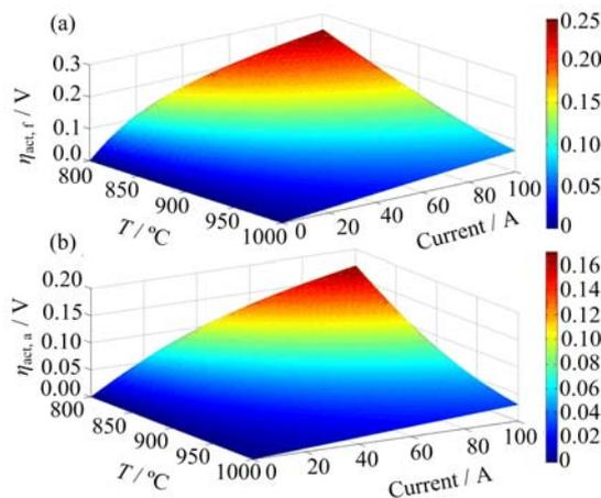
FIG. 2 Activation overpotentials in RSOC at 1 atm and 95% state of charge for the (a) fuel electrode and (b) air electrode, respectively.
