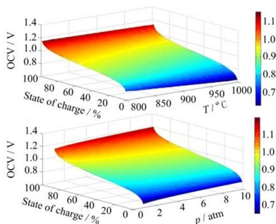
FIG. 1 The OCV of the RSOC system versus (a) temperature and (b) pressure in the state of charge (1%–99%).
