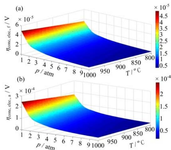
FIG. 3 Relationship between temperature, pressure and concentration overpotential in (a) fuel electrode and (b) air electrode at 1 A current and 95% state of charge in the fuel cell mode.
