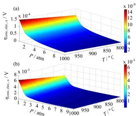
FIG. 4 Relationship between temperature, pressure and concentration overpotential in (a) fuel electrode and (b) air electrode at 1 A current and 95% state of charge in the electrolysis mode.
