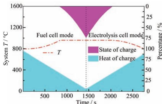
FIG. 6 Cycling performance of RSOC for the storage and utilization of electricity at 1 A per cell at the beginning conditions of 1 atm, 800 °C, and 95% state of charge.
