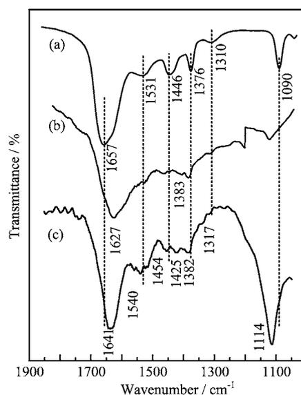
FIG. 6 FT-IR spectra of (a) aHA, (b) hematite, and (c) aHA-treated hematite.
