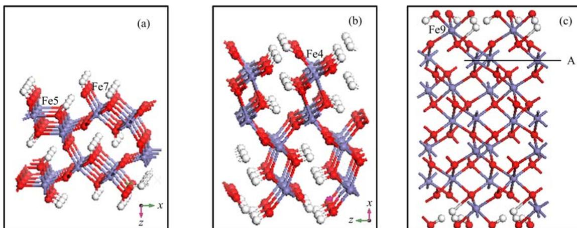
FIG. 3 Truncated side view of the model for (a) goethite (101), (b) goethite (100) and (c) hematite (001) surfaces. A horizontal line indicates a type-A termination is obtained by removing the atoms above the line. Oxygen atoms are shown in red, iron atoms in grayish blue and hydrogen atoms in white.
