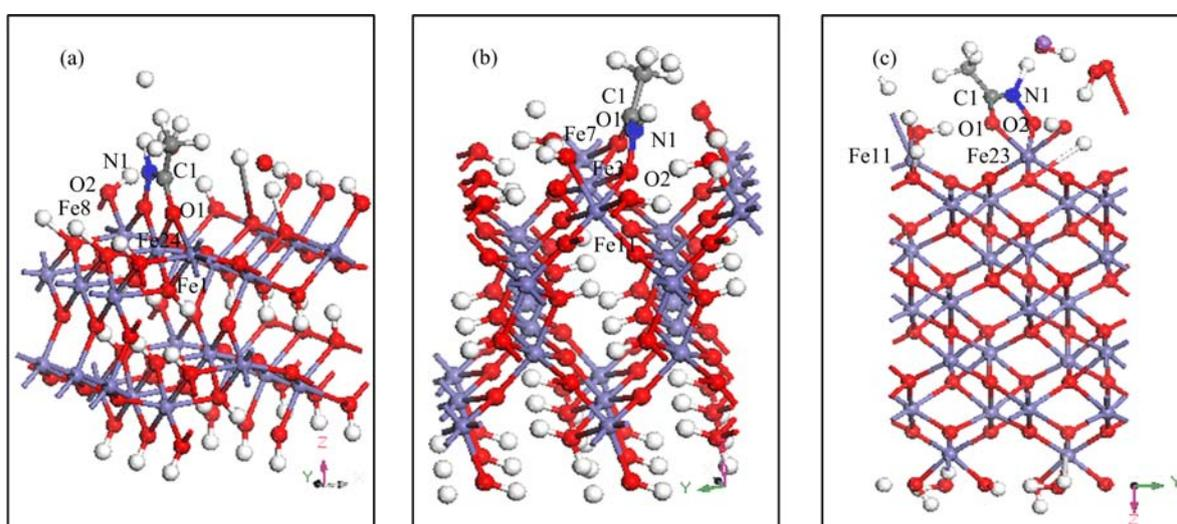
FIG. 4 Illustration of the optimized interfacial structures of aHA adsorbed on (a) goethite (101), (b) goethite (100), and (c) hematite (001) surface. Iron atoms are shown in purple, oxygen atoms in medium red, nitrogen atoms in blue and hydrogen atoms in white.
