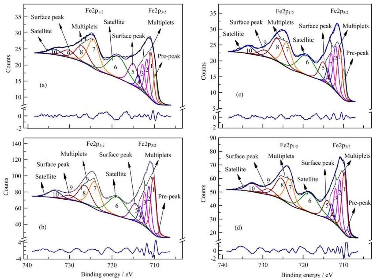
FIG. 7 The Fe2p spectra and the fitting curves of (a) goethite, (b) hematite, (c) aHA-treated goethite, and (d) aHA-treated hematite.
