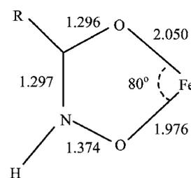
FIG. 8 Model compounds of  $[\text{Fe}(\text{aha})_3]$  ( $\text{aha}^-$  is acetohydroxamate) labeled with key interatomic distances in Å and the bond angle [36].
