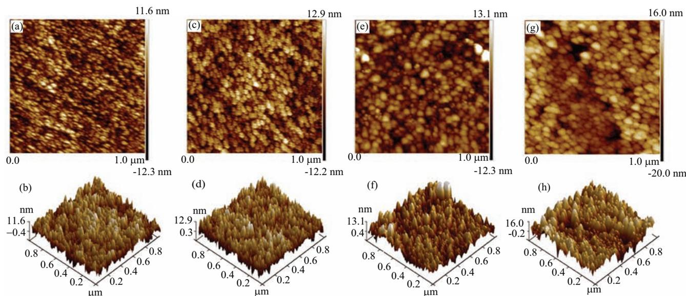
FIG. 2 Two- and three-dimensional AFM images of the BZO films deposited at (a, b) 350 °C, (c, d) 400 °C, (e, f) 450 °C, (g, h) 500 °C
