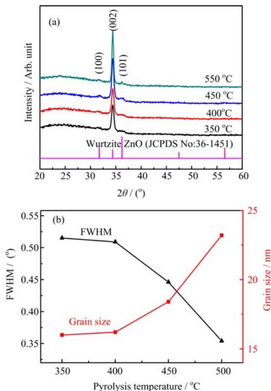
FIG. 1 (a) XRD  $2\theta$  scan patterns and (b) FWHM values and average crystallite sizes of the BZO films deposited at different pyrolysis temperatures.
