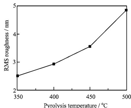
FIG. 3 RMS roughness of the BZO films deposited at different pyrolysis temperatures.
