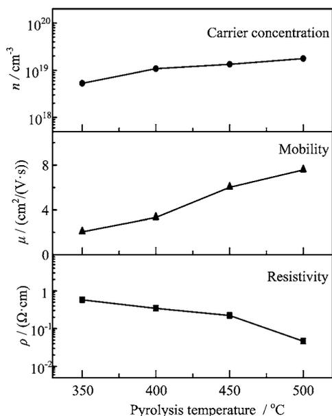
FIG. 4 Electrical properties of the BZO films as a function of the pyrolysis temperature.
