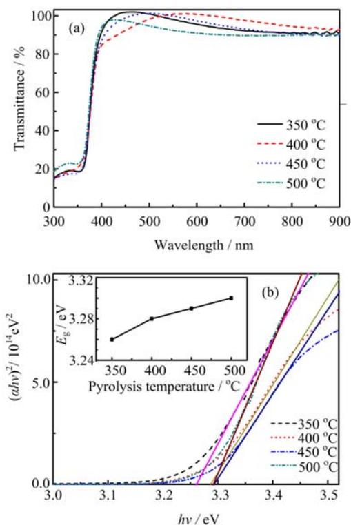
FIG. 5 (a) Transmittance spectra and (b)  $(\alpha h\nu)^2$  versus  $h\nu$  plot of the BZO films deposited at different pyrolysis temperatures. Inset: the optical band gap of the films.
