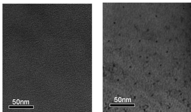
FIG. 6 TEM images of the PIS07 (left) and PIS15 (right) hybrid membranes.
