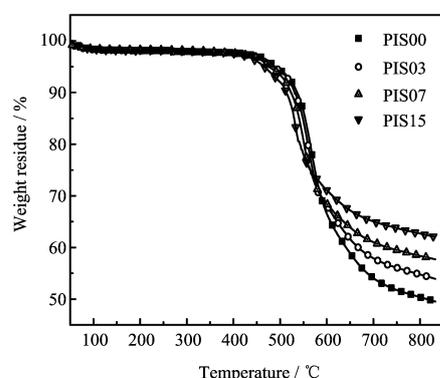
FIG. 5 Thermogravimetric profiles of the PIS00-15 hybrid materials.
