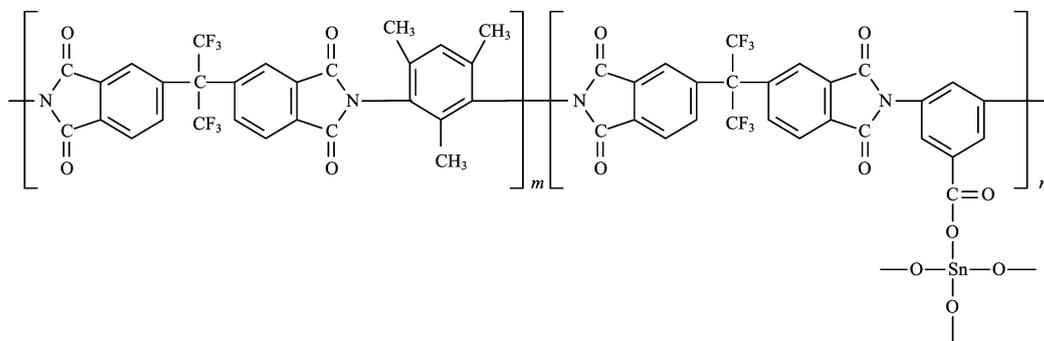
FIG. 4 The structure model of the polyimide/SnO<sub>2</sub> hybrid materials.
