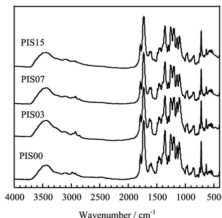
FIG. 1 FTIR spectra of the membrane materials.
