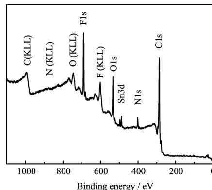
FIG. 2 XPS survey spectrum of the PIS07 hybrid membrane.
