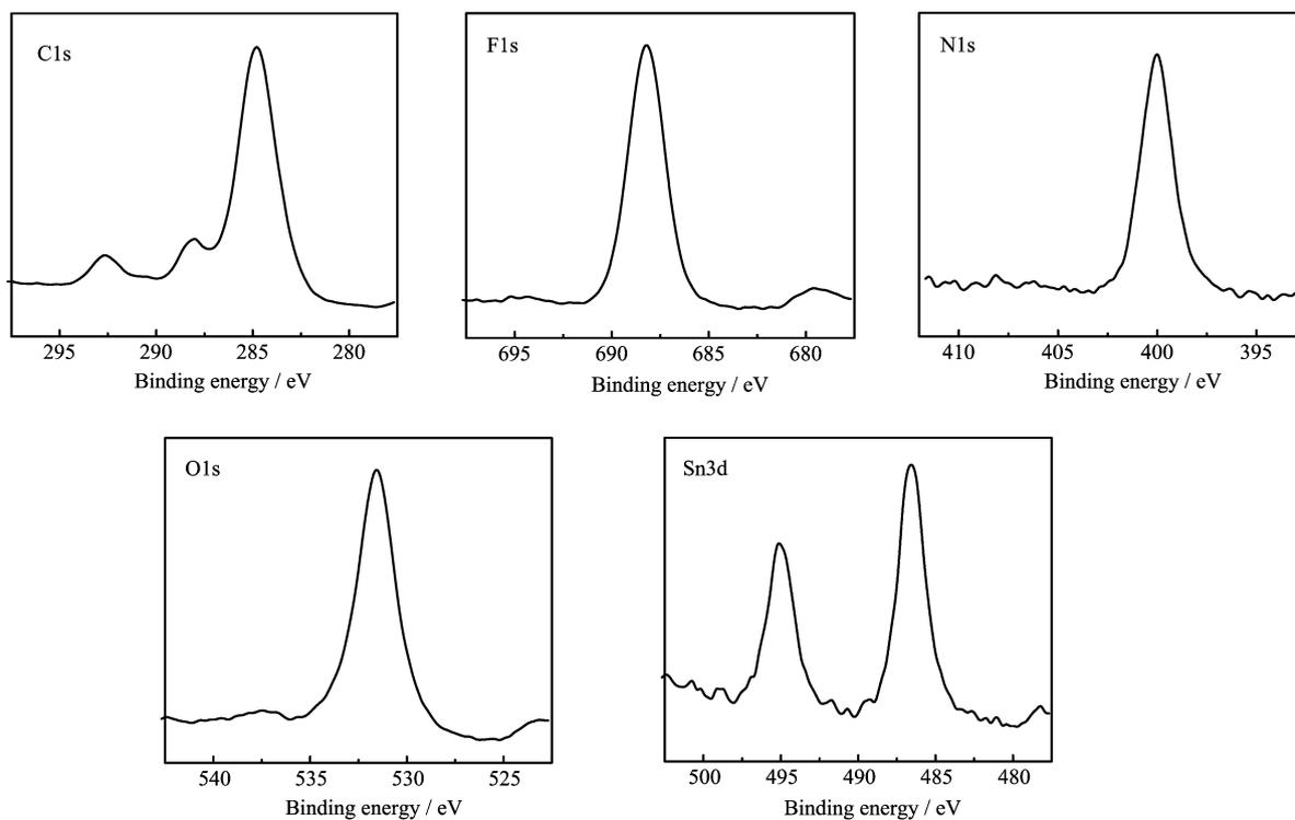
FIG. 3 XPS spectra of C1s, O1s, F1s, N1s and Sn3d in the PIS07 hybrid membrane.
