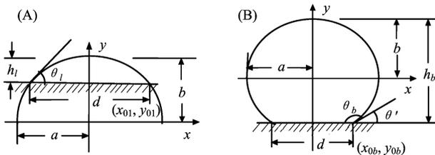
FIG. 1 The profile of droplet in the case of  $CA < 90^\circ$  in hydrophilic state (A); and in the hydrophobic state  $CA > 90^\circ$  (B).  $a$  and  $b$  are semi-axis lengths; the three parameters  $\theta_l$  ( $\theta_b$ ),  $d$  and  $h_l$  ( $h_b$ ) are the contact angle ( $CA$ ), contact diameter, and height of the droplet, respectively.
