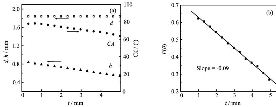
FIG. 2 (a) Evolution of  $CA$ ,  $d$  and  $h$  for a water droplet with initial volume of about  $1 \mu\text{L}$  on smooth PC surface in open air; (b) Plot of function  $F(\theta)$  in the spherical cap model against evaporation time  $t$ .
