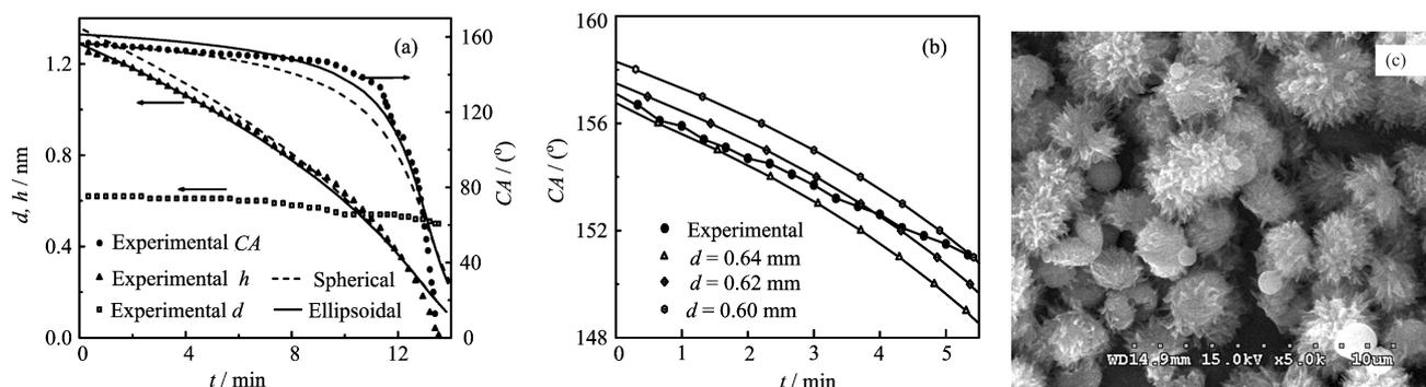
FIG. 3 (a) Evolution of  $CA$ ,  $d$  and  $h$  for a water droplet of initial volume about  $1 \mu\text{L}$  on superhydrophobic PC surface in open air. The scatter lines are the fitting curves of  $CA$  and  $h$  against evaporation time  $t$  based on ellipsoidal and spherical models; (b) Time dependence of  $CA$  from experimental data and calculated data with different radii; (c) SEM image of superhydrophobic PC surface with micro-nano-binary structure.
