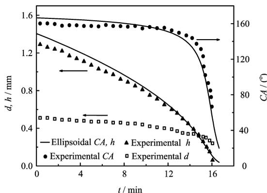
FIG. 4 Evolution of  $CA$ ,  $d$  and  $h$  for a water droplet of initial volume about  $1 \mu\text{L}$  on superhydrophobic FPU/PMMA surface in open air. The solid lines are fitting curves of  $CA$  and  $h$  against  $t$  based on the ellipsoidal model.
