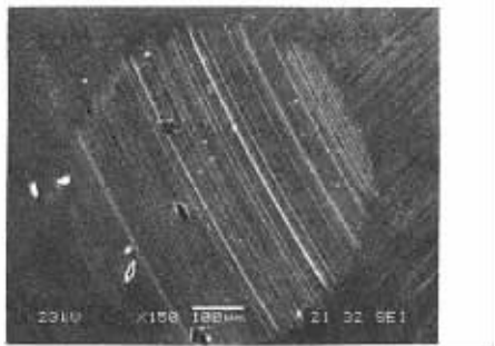
Fig. 6 SEM image of the rubbing surface lubricated by 0.5% Pb nanoparticles
