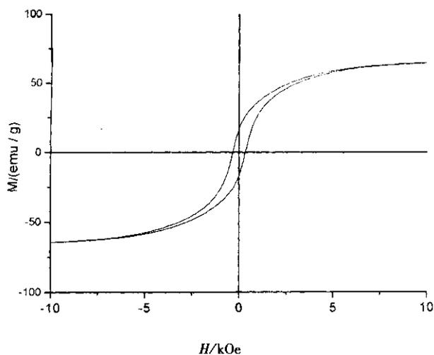
Fig. 3 M-H hysteresis loop of the products at room temperature
