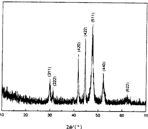
Fig. 1 XRD pattern of the as-prepared samples
