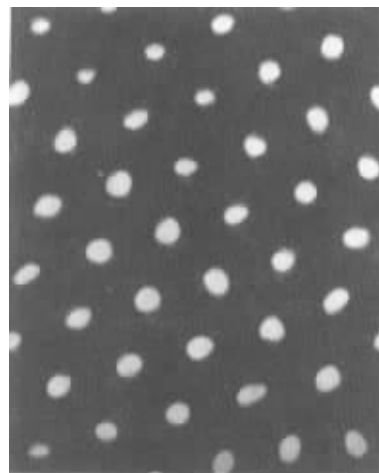
4 二次阳极氧化铝膜孔形貌的 TEM 照片 4 Plan-view TEM image of the anodic alumina film made by two-step anodization
