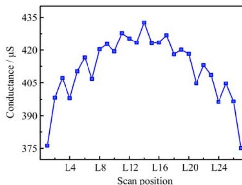
FIG. 3 The variation of the first conductance peak intensity with the AC container sliding from L1 to L27 in our AC@SWNT(5, 5) system.
