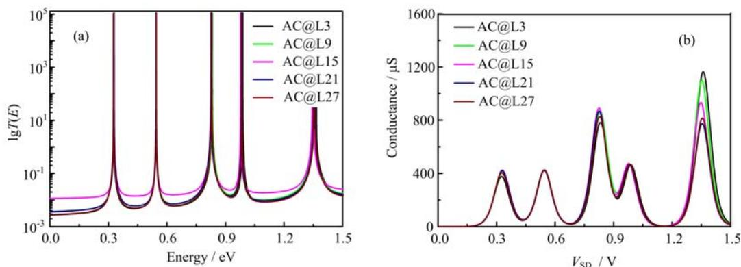
FIG. 2 (a) The computed electron transmission spectra in log scale and (b) conductance-voltage curves for the AC@SWNT(5, 5) system with AC attached to the L3, L9, L15, L21, L27 positions (named as AC@ $L_i$ ).
