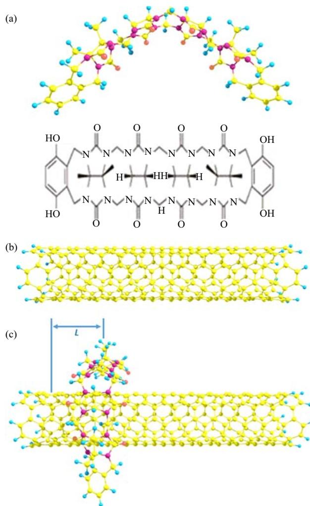
FIG. 1 (a) The atomic model (upper) and chemical structure (lower) of the AC molecular container. (b) The atomic model for a (5, 5) armchair SWNT. (c) The schematic illustration of the electronic conductance measurement setup for the designed AC@SWNT(5, 5) structure (SWNT encapsulated by AC). Here the yellow, blue, purple, and red beads stand for C, H, N, and O atoms, respectively.
