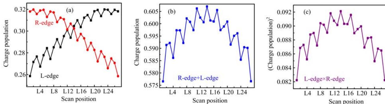
FIG. 4 The computed edge charge populations of (a) left edge (L-edge) and right edge (R-edge), (b) charge summation of L-edge+R-edge, and (c) charge product of L-edge $\times$ R-edge in the first conducting channel (corresponding to the first peak in the conductance curve) of AC@SWNT(5, 5).
