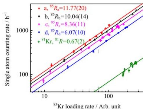
FIG. 3 Ratio between the  $^{85}\text{Kr}$  counting rate and the  $^{83}\text{Kr}$  loading rate measured by the ATTA-Hefei setup. Four commercial krypton gas samples were used, referred as samples a, b, c, and d. Samples a and c were produced in 2012 and 2007 respectively.
