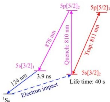
FIG. 1 Energy levels and transitions related to the ATTA measurement of Kr.
