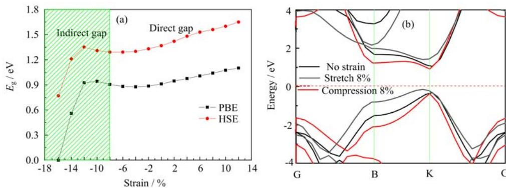
FIG. 4 (a) The band gap and (b) band structures of BP monolayer under a uniaxial strain.
