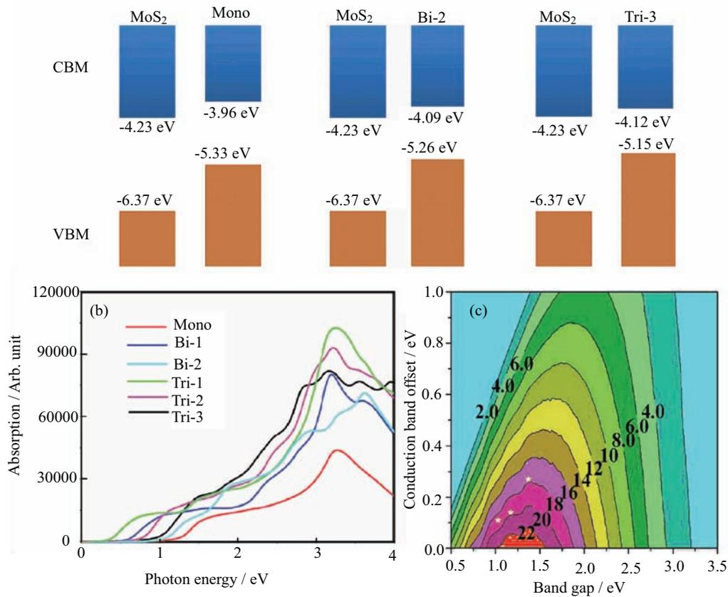
FIG. 3 (a) The band alignment of MoS<sub>2</sub>/BP van der Waals heterojunctions. (b) The optical absorption spectra of BP layers. (c) The computed PCE as a function of donor band gap and conduction band offset.
