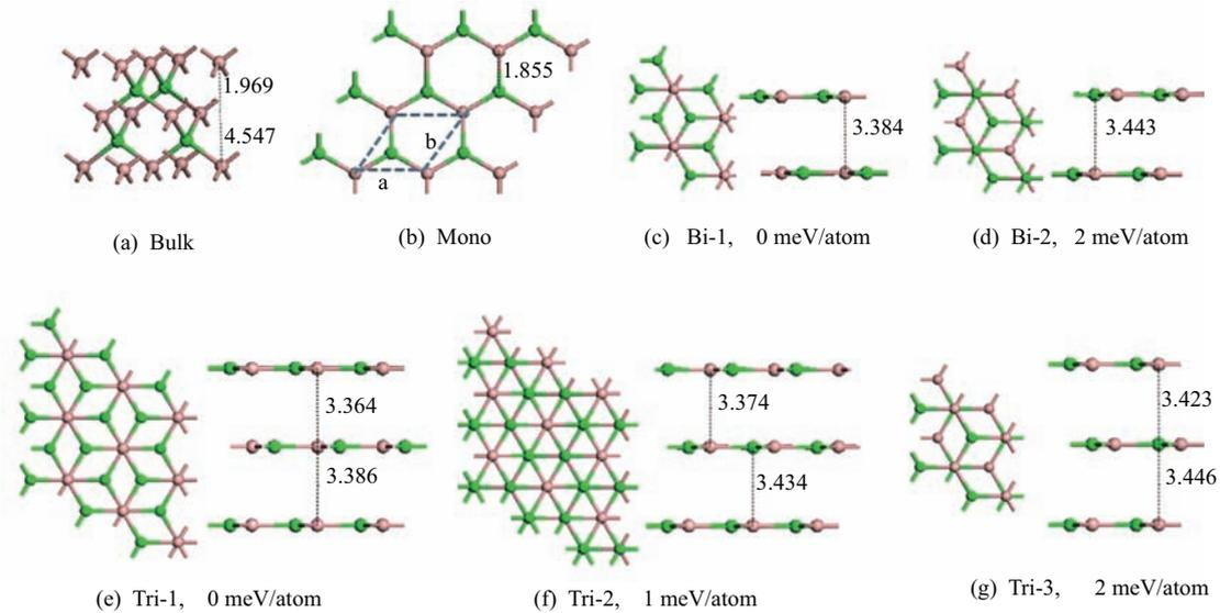
FIG. 1 The optimized structures of (a) BP bulk, (b) BP monolayer, (c) and (d) BP bilayer with AA and AB stacking, respectively, and (e)–(g) BP triple-layers with AAA, AAB and ABA stacking, respectively. Pink and blue ball denote boron and phosphorus atom, respectively.
