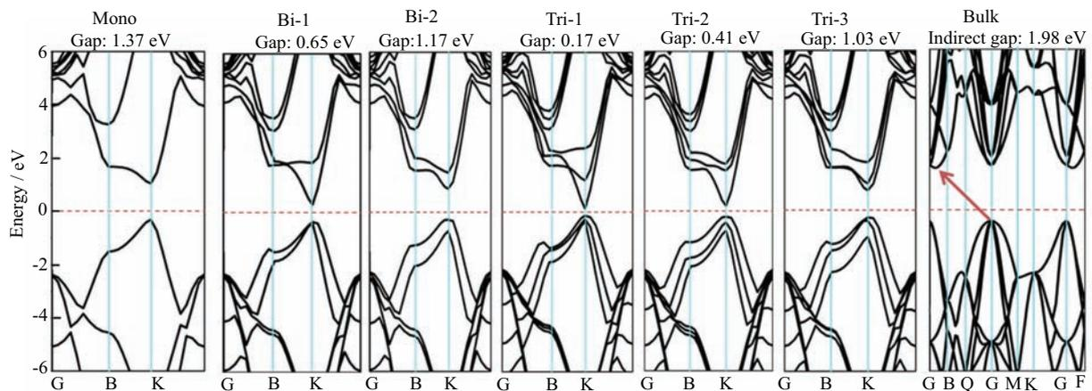
FIG. 2 The calculated electronic band structures of graphene-like BP monolayer, bilayer (Bi-1 and Bi-2) and tri-layer (Tri-1, Tri-2, and Tri-3), and zinc blende bulk BP.
