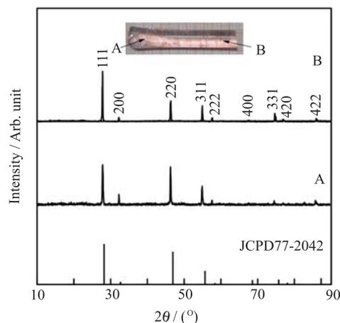
FIG. 1 XRD patterns of  $\text{Ho}^{3+}/\text{Yb}^{3+}$  co-doped  $\alpha\text{-NaYF}_4$  single crystal of different part. Insert is the photo of  $\alpha\text{-NaYF}_4$  single crystal.
