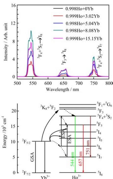
FIG. 2 (a) Comparison of the upconversion luminescence spectra of  $\text{Ho}^{3+}/\text{Yb}^{3+}$  codoped  $\alpha\text{-NaYF}_4$  single crystals under 980 nm excitation at room temperature. (b) Energy level diagram of  $\text{Ho}^{3+}/\text{Yb}^{3+}$  upconversion and energy transfer process in  $\alpha\text{-NaYF}_4$  single crystal.
