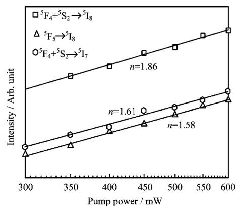
FIG. 3 lg-lg dependences of the upconversion intensities of 0.998mol% Ho<sup>3+</sup> and 8.08mol% Yb<sup>3+</sup> co-doped  $\alpha$ -NaYF<sub>4</sub> single crystal at 544, 657, and 751 nm emissions as a function of the excitation power at 980 nm.
