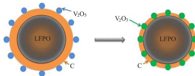
FIG. 1 Schematic illustration for the formation of the  $\text{V}_2\text{O}_3$ -C dual-layer coated on the  $\text{LiFePO}_4$  particles by carbothermic reduction of  $\text{V}_2\text{O}_5$ .
