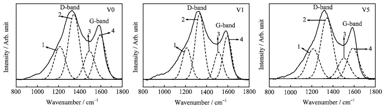
FIG. 4 Raman spectra of V0, V1, and V5. 1:  $1194\text{ cm}^{-1}$ , 2:  $1347\text{ cm}^{-1}$ , 3:  $1510\text{ cm}^{-1}$ , 4:  $1585\text{ cm}^{-1}$ .
