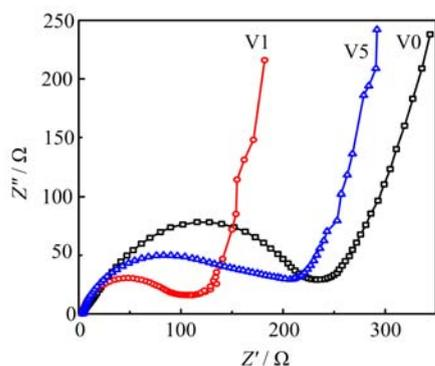
FIG. 6 Nyquist plots of the cells using V0, V1, and V5 after the initial cycle.
