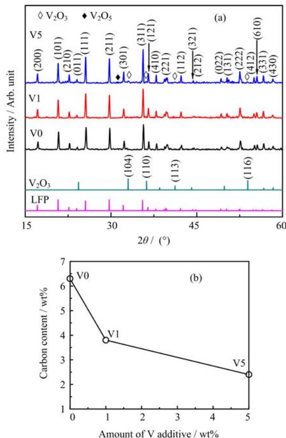
FIG. 2 (a) XRD pattern of the V<sub>2</sub>O<sub>3</sub>-C dual-layer coated on the LiFePO<sub>4</sub> nanoparticles and (b) the relationship of carbon content *vs.* vanadium oxide content.
