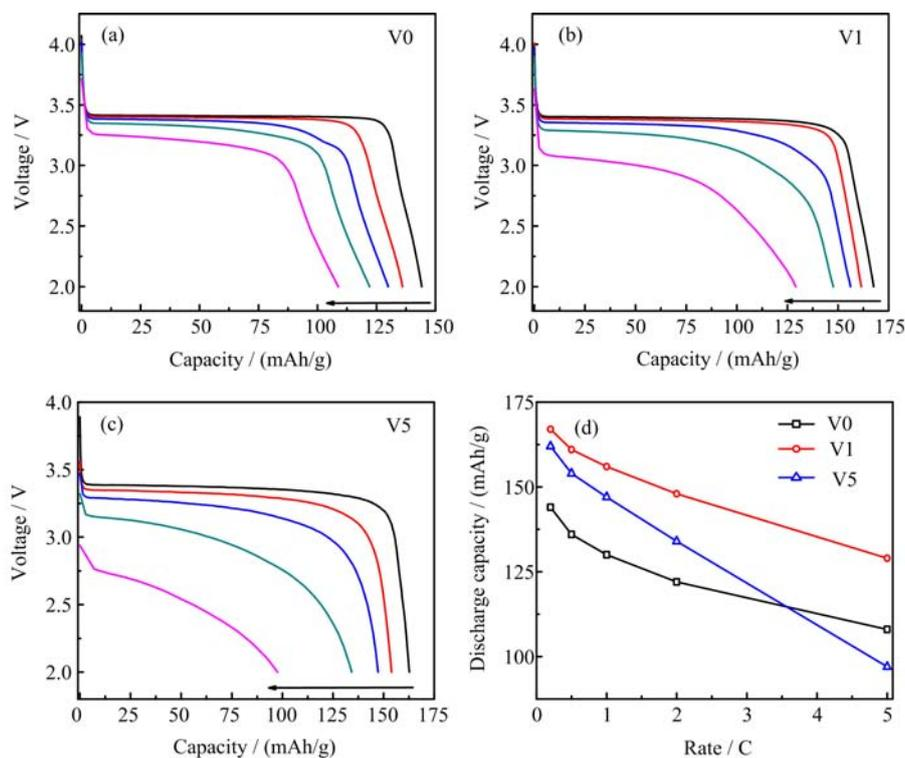
FIG. 8 Rate discharge curves of the cells using (a) V0, (b) V1, and (c) V5 at 0.2, 0.5, 1, 2, 5 C rates, as arrows show. (d) Discharge capacity values.
