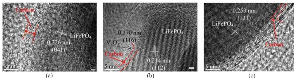
FIG. 3 HRTEM images of (a) V0, (b) V1, and (c) V5.
