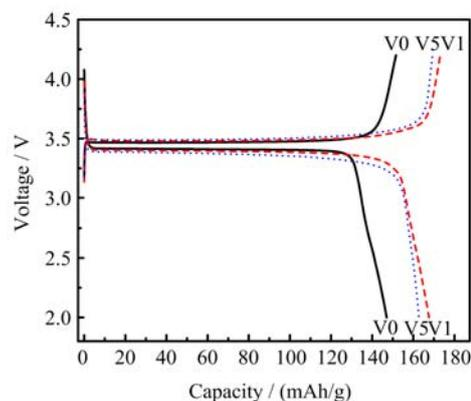
FIG. 5 Initial charge and discharge capacities of the cells using V0, V1, and V5 at  $0.2\text{ C}$ .
