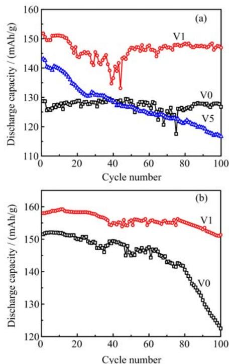
FIG. 7 Cycling performance of the cells using V0, V1 and V5 at 1 C at (a) 25 °C and (b) 55 °C.
