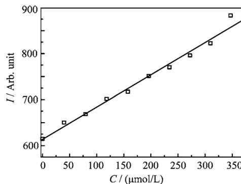
FIG. 7 Dependence of the fluorescence intensity of the PU/HgS film on concentration of Ba<sup>2+</sup>.
