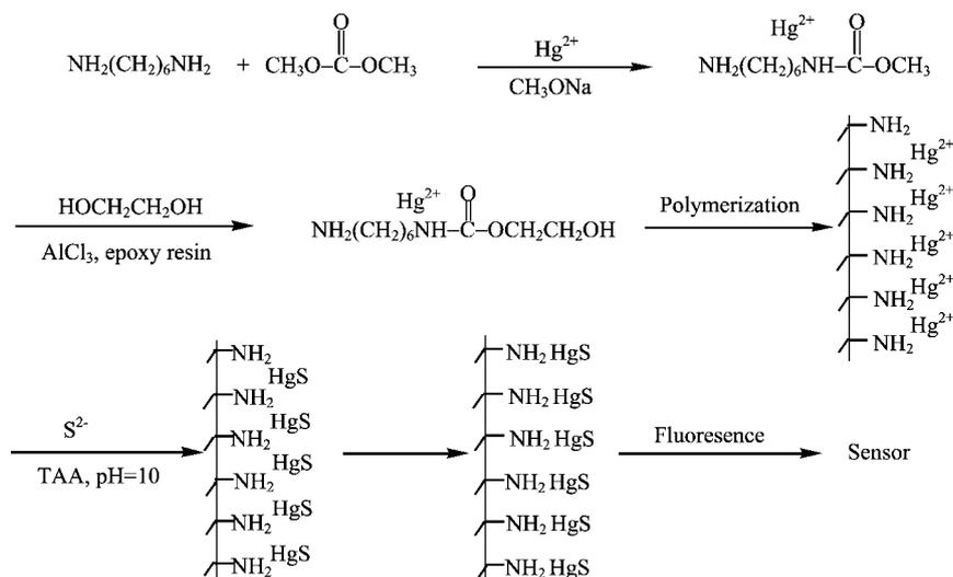
FIG. 1 Schematic of PU/HgS nanocomposite film.
