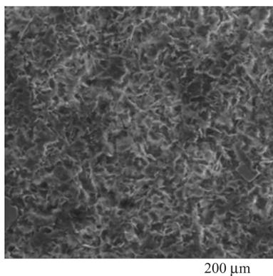
FIG. 4 SEM of PU/HgS film.
