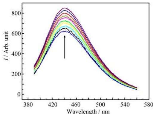
FIG. 6 The fluorescence property of PU/HgS film in various concentrations of Ba<sup>2+</sup> from 0, 39.8, 79.36, 118.58, 157.48, 196.07, 234.37, 272.37, 310.1, to 347.1  $\mu\text{mol/L}$  as arrow shows.
