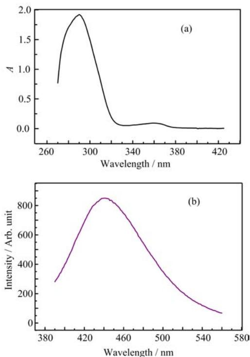
FIG. 2 (a) UV-Vis spectrum and (b) fluorescence emission spectrum of the PU/HgS nanocomposite film.
