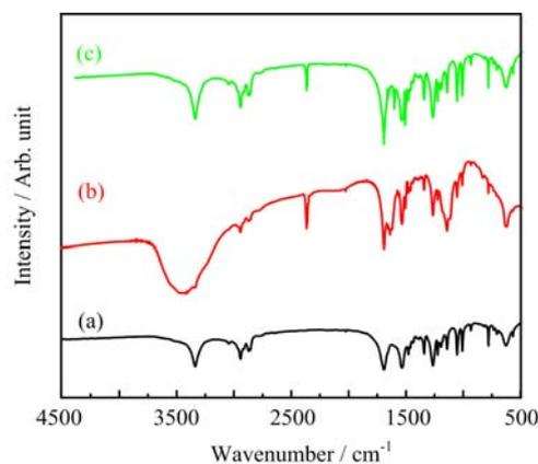
FIG. 3 FTIR spectral data of (a) PU, (b) intermediate, and (c) PU/HgS film.
