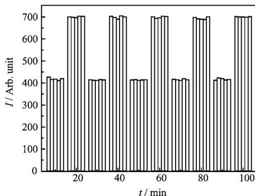
FIG. 8 Reversibility of the film sensor for Ba<sup>2+</sup>.
