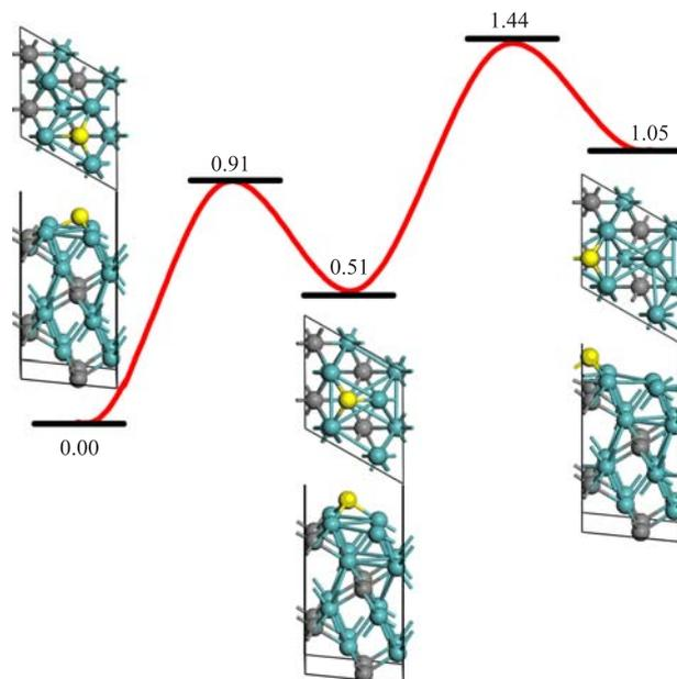
FIG. 6 Diffusion of C adatom (highlighted in yellow) on the (001) surface from O-site to T-site and then C-site. Relative energies compared to the most stable adsorption structure are given in eV.
