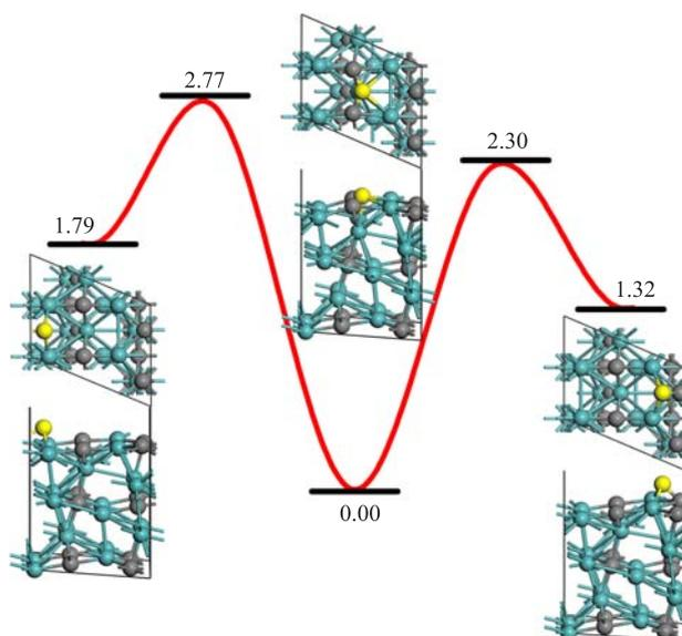
FIG. 7 Diffusion of C adatom (highlighted in yellow) on the (101) surface in the [100] direction. Relative energies compared to the most stable adsorption structure are given in eV.
