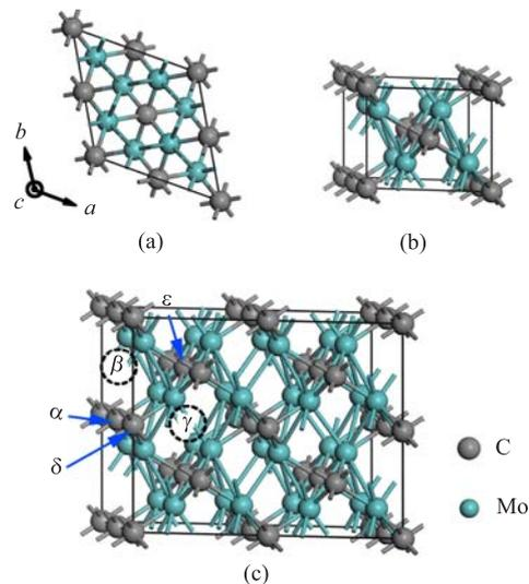
FIG. 1 (a) Top view and (b) side view of  $\text{Mo}_2\text{C}$  unit cell. (c) A  $2\times 1\times 2$  supercell with some atomic sites marked.
