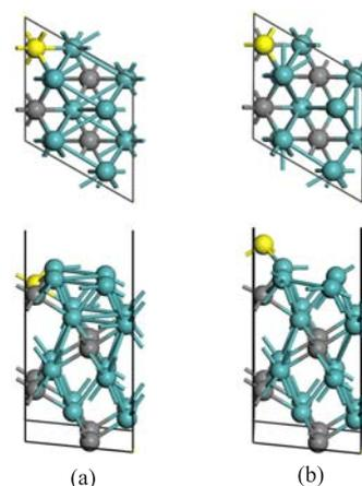
FIG. 4 (a) The  $\text{Mo}_2\text{C}(001)$  surface and (b) the corresponding structure with a surface C atom lifted up as an adatom. This atom is highlighted in yellow. For both structures, top view is shown in the upper panel and side view is shown in the down panel.
