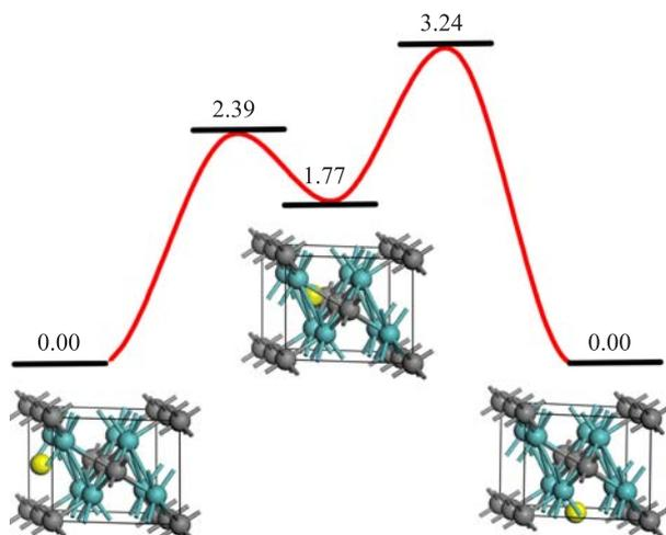
FIG. 3 The diffusion pathway of a C dopant (highlighted in yellow) in  $\text{Mo}_2\text{C}$  bulk from site  $\beta$  to site  $\gamma$ . Energy is given in eV. Geometries of the initial, intermediate, and final states are illustrated in a  $1 \times 1 \times 1$  unit cell.
