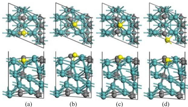
FIG. 5 (a) The  $\text{Mo}_2\text{C}(101)$  surface and (b) the corresponding structure with a surface C atom lifted up as an adatom. This atom is highlighted in yellow. (c) The most stable structure of a C adatom on the (101) surface and (d) the structure with the C adatom moved to a neighboring adsorption site in the [010] direction. For all structures, top view is shown in the upper panel and side view is shown in the down panel.
