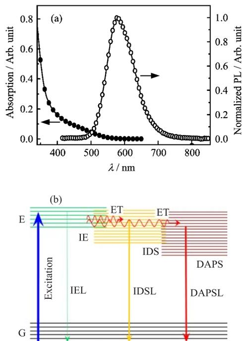
FIG. 1 (a) UV-Vis absorption and photoluminescence spectra of ZnCuInS/ZnSe/ZnS QDs. (b) Proposed luminescence mechanism in ZnCuInS/ZnSe/ZnS QDs. IE: intrinsic exciton, IEL: intrinsic exciton luminescence, IDS: the interface defect state luminescence, DAPSL: the donor-acceptor pair state luminescence, ET: energy transfer; E: excited state; G: ground state.
