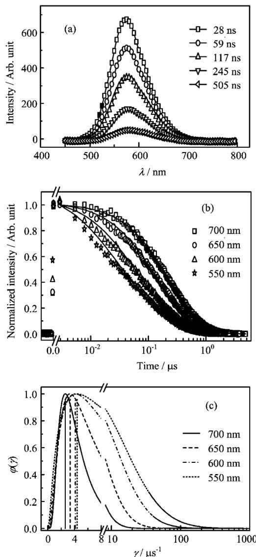
FIG. 2 (a) The temporal emission spectra of quantum dots. (b) Wavelength-dependent emission curves. (c) The decay-rate distributions  $\varphi(\gamma)$  at different wavelengths.  $\gamma_{MF}$  of emission traces at 550, 600, 650, and 700 nm are 4.39, 4.13, 3.33, and  $2.62 \mu\text{s}^{-1}$ , and the widths ( $\Delta\gamma$ ) of their distribution function are 26.00, 16.97, 8.94, and  $5.10 \mu\text{s}^{-1}$ .
