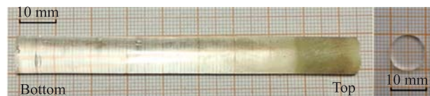
FIG. 1 \text{Tm}^{3+}/\text{Yb}^{3+} codoped \text{LiYF}_4 single crystal (left) and polished crystal (right).
