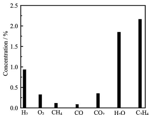
FIG. 8 Product distribution in ODH of ethane, at 650 °C, from experiments using the BSCF membrane reactor. Reactant side: 40.5% $C_2H_6$  (10 mL/min), feed side:  $p_{O_2}=0.80$  atm.
