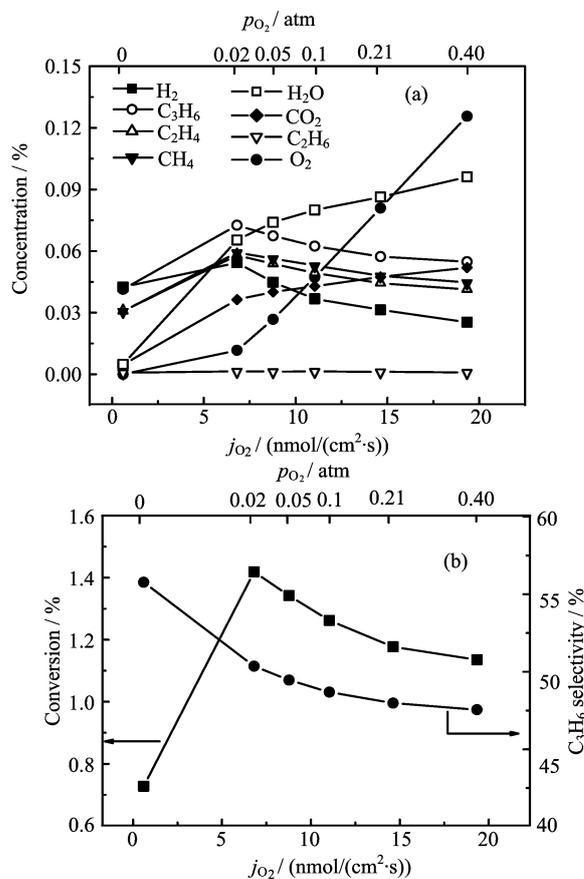
FIG. 7 Catalytic performance of the BSCF membrane reactor in ODH of propane, at 550 °C, as a function of the oxygen permeation flux. (a) Product distribution and (b) conversion and propylene selectivity. Reactant side: 10% $C_3H_8$  (10 mL/min).
