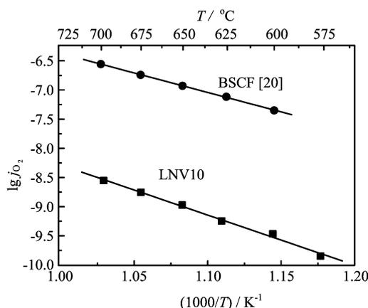
FIG. 3 Oxygen permeation flux ( $j_{O_2}$ ) through a disc LNV10 membrane with thickness 0.97 mm. Synthetic air was used as feed gas (100 mL/min), while helium was used as purge gas (10 mL/min) at the permeate side of the membrane. Also shown are data for a BSCF membrane with thickness of 1.5 mm from Ref.[20].
