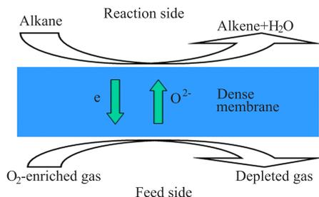
FIG. 1 Schematics of catalytic membrane reactor.
