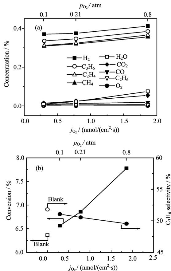
FIG. 5 Catalytic performance of the LNV10 membrane reactor in ODH of propane, at 650 °C, as a function of the oxygen permeation flux ( $j_{O_2}$ ). (a) Product distribution and (b) conversion and propylene selectivity. Reactant side: 10% $C_3H_8$  (10 mL/min). Oxygen partial pressures maintained at the feed side of the membrane are indicated in the figures. Also indicated in (b) are corresponding results from propane pyrolysis experiments (blank), at 650 °C, performed in an empty quartz reactor.
