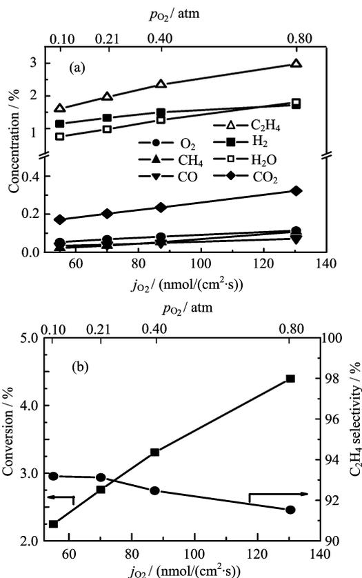
FIG. 9 Catalytic performance of the BSCF membrane reactor in ODH of ethane, at 650 °C, as a function of the oxygen permeation flux. (a) Product distribution and (b) conversion and ethylene selectivity. Reactant side: 73.9% $C_2H_6$  (10 mL/min). Oxygen partial pressures maintained at the feed side of the membrane are indicated in the figures.
