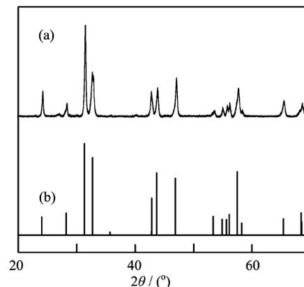
FIG. 2 X-ray powder diffraction pattern of (a) LNV10 collected at room temperature and (b) the calculated pattern.
