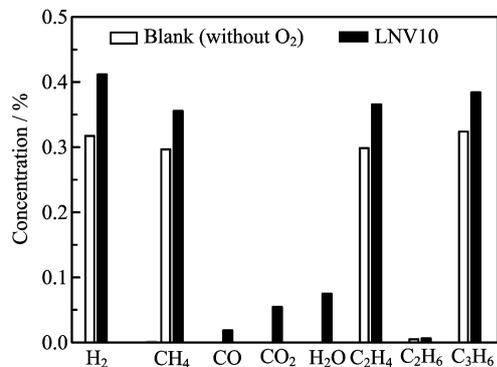
FIG. 4 Product distribution in ODH of propane, at 650 °C, from experiments using the LNV10 membrane reactor. Reactant side: 10% $C_3H_8$  (10 mL/min), feed side:  $p_{O_2}=0.80$  atm. Also shown are corresponding results of propane pyrolysis experiments (blank), at 650 °C, performed in an empty quartz reactor.
