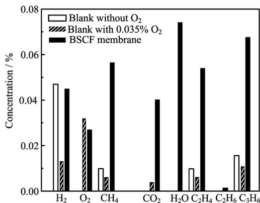
FIG. 6 Product distribution in ODH of propane, at 550 °C, from experiments using the BSCF membrane reactor. Reactant side: 10% $C_3H_8$  (10 mL/min), feed side:  $p_{O_2}=0.05$  atm. Also shown are corresponding data of thermal pyrolysis experiments (blank, without  $O_2$ ) and ODH of propane (blank, with  $O_2$ ), at 550 °C, performed in an empty quartz reactor.
