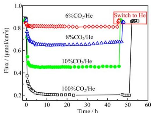
FIG. 6 Time dependence of oxygen permeation flux through SCFM membrane in a sweep gas containing different content of CO<sub>2</sub>. It is also shown that the permeation flux is totally recovered quickly when CO<sub>2</sub> is removed from the sweep gas.
