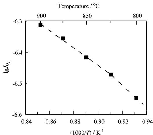
FIG. 4 Arrhenius plot of oxygen permeation flux through SCFM membrane under air/He gradient. Membrane thickness=1.0 mm.
