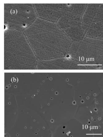
FIG. 2 SEM images of sintered SCFM membrane. (a) Surface and (b) cross-section.
