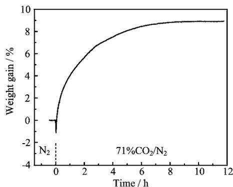
FIG. 5 Weight change of SCFM powder upon exposure to 71% CO<sub>2</sub> at 900 °C.
