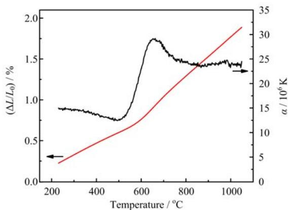
FIG. 3 Thermal expansion behavior of SCFM.
