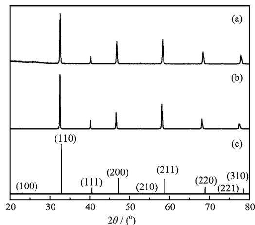
FIG. 1 XRD patterns of different sample. (a) SCFM powder calcined at 950 °C for 10 h, (b) SCFM membrane sintered at 1230 °C for 5 h, and (c) standard pattern of  $\text{SrCo}_{0.81}\text{Fe}_{0.19}\text{O}_{2.78}$  (JCPDS No.82-2445).
