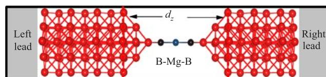
FIG. 1 The MgB<sub>2</sub> linear atomic chain attached to Au(100)-3×3 leads.
