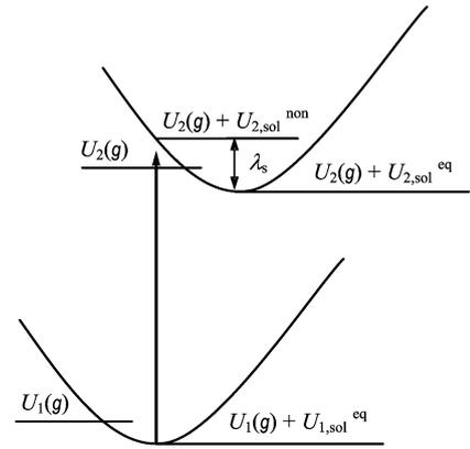
FIG. 2 A generic schematic depiction of solvent effect of absorption spectra in aqueous solution.
