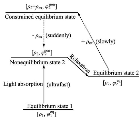
FIG. 1 A generic schematic diagram for the constrained equilibrium approach.
