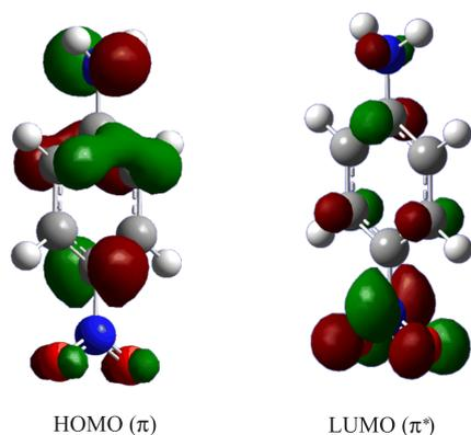
FIG. 4 HOMO and LUMO frontier orbitals involved in the lowest  $\pi \rightarrow \pi^*$  electronic transition.
