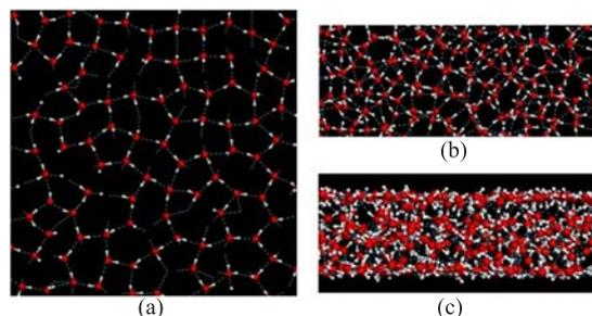
FIG. 5 Inherent structure obtained from MD simulation at  $d=1.2$  nm and  $P_L=1$  GPa. (a) The top view of the upper layer of this amorphous structure. (b) The zoomed top view of the amorphous. (c) The side view of the amorphous. Oxygen atoms are depicted in red, hydrogen atoms in white, and hydrogen bonds in blue dotted lines.
