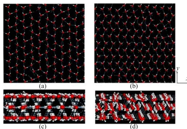
FIG. 4 Inherent structure of fhRTI obtained from MD simulation at  $d=1.0$  nm and  $P_L=1$  GPa. (a, b) Top view of the ice layer next to one of the walls and at the middle slab. (c, d) Side view of fhRTI at direction of  $x$  and  $y$ . Oxygen atoms are depicted in red, hydrogen atoms in white, and hydrogen bonds in blue dotted lines.
