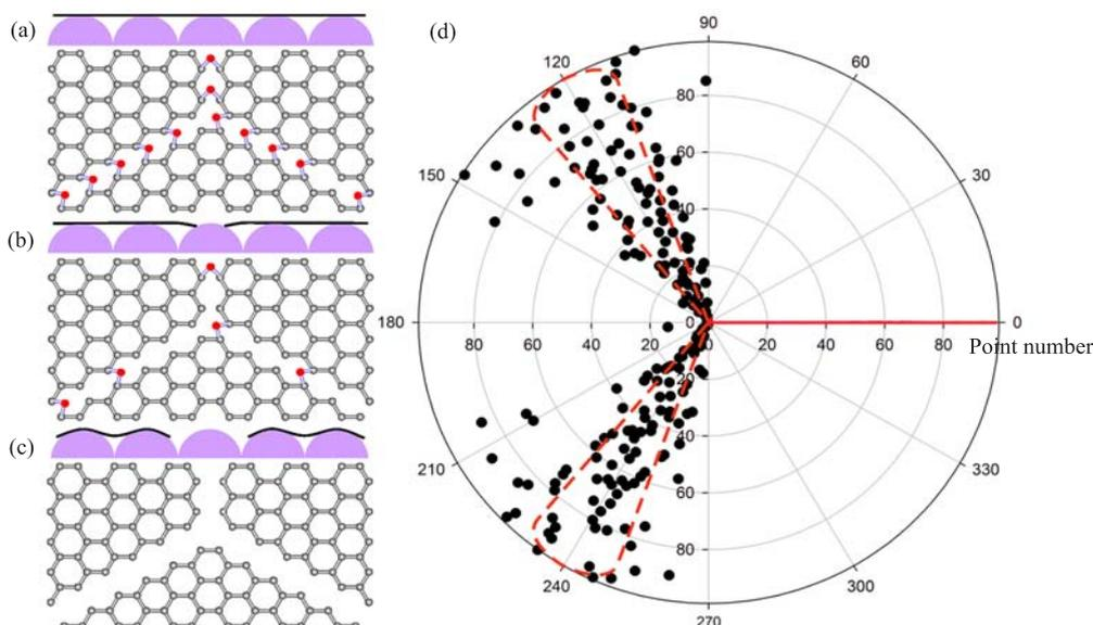
FIG. 4 (a)–(c) The schematic illustration of cracking process of GO sheets through unzipping along the aligned linear epoxy groups and formed three cracking small GO pieces. (d) Statistical results of the angular vertex of adjacent pieces of Fig.1(d).
