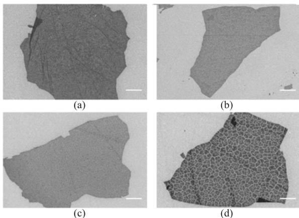
FIG. 1 SEM images of GO coated on the as-prepared (a, b) and annealed (c, d) ZnO film after drying in atmosphere for 3 h (a, c) and 10 h (b, d). The scale bar is 4  $\mu\text{m}$ .
