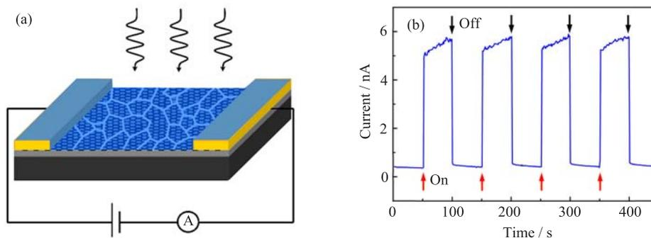
FIG. 5 (a) The schematic diagram of the device. (b) The photoresponse of the devices at 1.0 V bias voltage under the white light with power density of  $100 \text{ mW/cm}^2$ .
