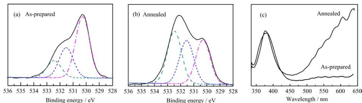
FIG. 3 XPS of O1s (a) the as-prepared and (b) the annealed ZnO films. (c) The corresponding PL results of two ZnO films.
