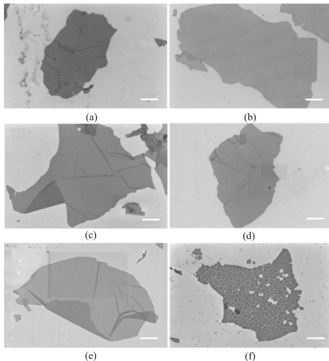
FIG. 2 SEM images of GO sheets on (a) Si, (b) 300 nm  $\text{SiO}_2$ , (c) 5 nm Au, (d) 100 nm ITO, (e) LCMO film, and (f) the transferred c-GO on  $\text{SiO}_2$  substrate. The scale bar is 4  $\mu\text{m}$ .
