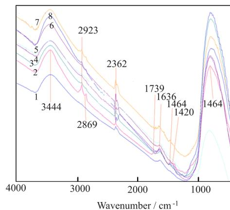
FIG. 4 IR spectra measured before and after hydrogen adsorption upon the Ni/Al<sub>2</sub>O<sub>3</sub> nano-composite at different temperatures (the different spectra are obtained: 1 before hydrogen adsorption; 2 at 25 °C and 40 bar, 3 at 75 °C and 20 bars; 4 at 75 °C and 40 bar, 5 at 150 °C and 20 bars, 6 at 150 °C and 40 bar, 7 at 300 °C and 40 bar, 8 at 300 °C and 20 bars.)
