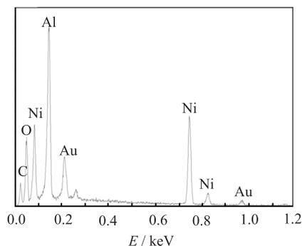
FIG. 2 EDX spectrum of  $\text{Ni}/\text{Al}_2\text{O}_3$  nano-composite.
