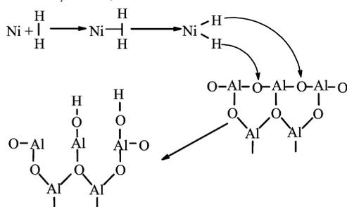
FIG. 6 Schematic representation of  $Al_2O_3$  network rupturing at  $300\text{ }^\circ\text{C}$ .
