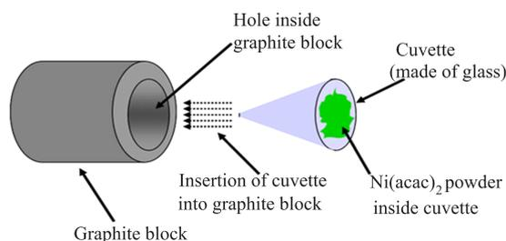
FIG. 1 Specially designed cuvette used for reduction of Ni(acac)<sub>2</sub> under flow of [H<sub>2</sub>Al(O<sup>t</sup>Bu)]<sub>2</sub>.
