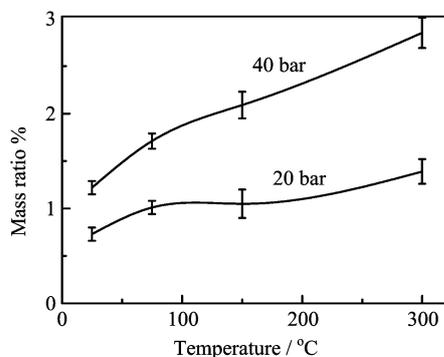
FIG. 3 Hydrogen adsorption as a function of temperature upon Ni/Al<sub>2</sub>O<sub>3</sub>.
