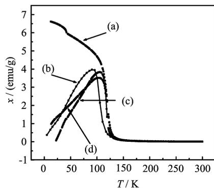
FIG. 3 Magnetic susceptibility plots as a function of temperature of  $\text{Pr}_{1-x}\text{Rb}_x\text{MnO}_3$ . (a)  $\text{Pr}_{0.92}\text{Rb}_{0.08}\text{MnO}_3(\text{FC})$ , (b)  $\text{Pr}_{0.95}\text{Rb}_{0.05}\text{MnO}_3(\text{ZFC})$ , (c)  $\text{Pr}_{0.92}\text{Rb}_{0.08}\text{MnO}_3(\text{ZFC})$ , (d)  $\text{Pr}_{0.94}\text{Rb}_{0.06}\text{MnO}_3(\text{ZFC})$ .
