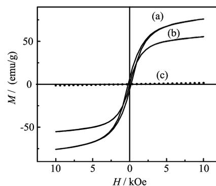
FIG. 5  $M$ - $H$  loops at different temperatures for  $\text{Pr}_{0.92}\text{Rb}_{0.08}\text{MnO}_{3.02}$ . (a) 5 K, (b) 80 K, and (c) 250 K.
