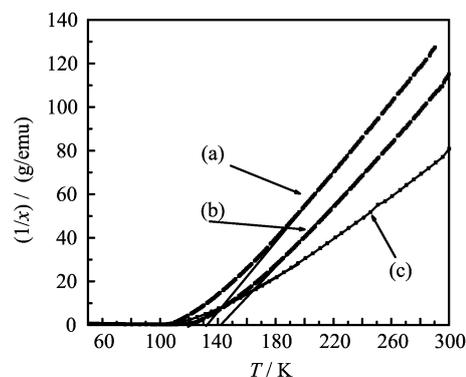
FIG. 4 inverse susceptibility plots as a function of temperature of  $\text{Pr}_{1-x}\text{Rb}_x\text{MnO}_3$ . (a)  $\text{Pr}_{0.94}\text{Rb}_{0.06}\text{MnO}_3$ , (b)  $\text{Pr}_{0.92}\text{Rb}_{0.08}\text{MnO}_3$ , and (c)  $\text{Pr}_{0.95}\text{Rb}_{0.05}\text{MnO}_3$ .
