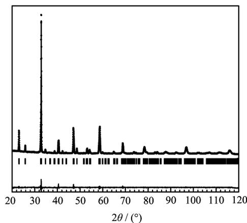
FIG. 2 Observed (dots), calculated (solid line) and difference (bottom) XRD patterns for Pr<sub>0.92</sub>Rb<sub>0.08</sub>MnO<sub>3.02</sub>.
