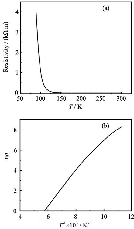
FIG. 6 (a) Temperature dependence of the resistivity for Pr<sub>0.92</sub>Rb<sub>0.08</sub>MnO<sub>3.02</sub>. (b)  $\ln\rho$  dependence of  $T^{-1}$  for Pr<sub>0.92</sub>Rb<sub>0.08</sub>MnO<sub>3.02</sub>.
