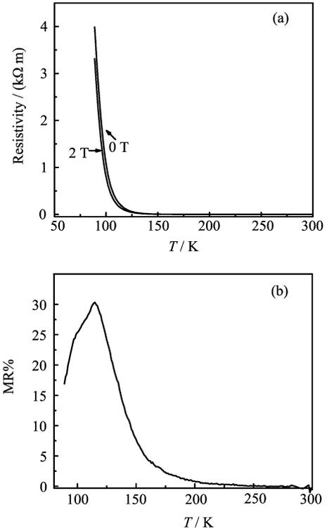
FIG. 7 (a) Temperature dependence of the resistivity for Pr<sub>0.92</sub>Rb<sub>0.08</sub>MnO<sub>3.02</sub> at 0 and 2 T magnetic fields. (b) The plot of MR% vs.  $T$  of Pr<sub>0.92</sub>Rb<sub>0.08</sub>MnO<sub>3.02</sub>.
