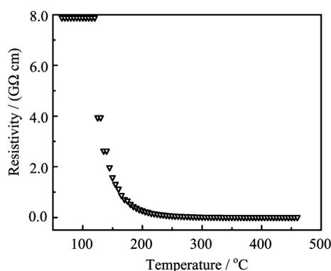
FIG. 4 Temperature-dependent DC electrical resistivity of  $\text{Zn}_{0.95}\text{Mn}_{0.05}\text{O}$ .
