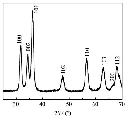
FIG. 1 XRD spectrum of  $\text{Zn}_{0.95}\text{Mn}_{0.05}\text{O}$ .
