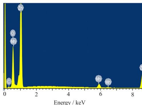
FIG. 2 EDX spectrum of  $\text{Zn}_{0.95}\text{Mn}_{0.05}\text{O}$ .
