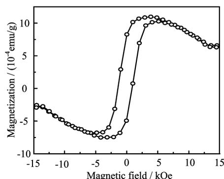
FIG. 5 Field dependent magnetization of  $\text{Zn}_{0.95}\text{Mn}_{0.05}\text{O}$ .
