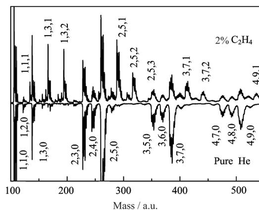
FIG. 1 TOF mass spectra for reaction of  $Zr_xO_y^+$  with  $C_2H_4$  in the fast flow reactor. The mass spectra with 2%  $C_2H_4$  and without  $C_2H_4$  being seeded in the helium carrier gas are given in the up and down panels, respectively. 1%  $O_2$  in 500 kPa helium is used to generate the clusters. Symbols  $x$ ,  $y$ ,  $z$  denote the mass spectrometer detected species  $Zr_xO_y(C_2H_4)_z^+$ .
