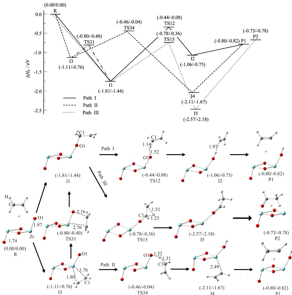
FIG. 3 Calculated potential energy profile of  $\Delta H_{0K}$  for reactions of  $\text{Zr}_2\text{O}_4^+$  with  $\text{C}_2\text{H}_4$ . The reaction intermediates and transition states are denoted as  $I_i$  and  $\text{TS}_{ij}$ , respectively. Energies for each species are given in the brackets as the form  $(\Delta H_{0K}/\Delta G_{298K})$ . Distances denoted by dashed line are given in Å.
