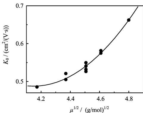
FIG. 5 Dependence of reduced mobility on ionic mass.
