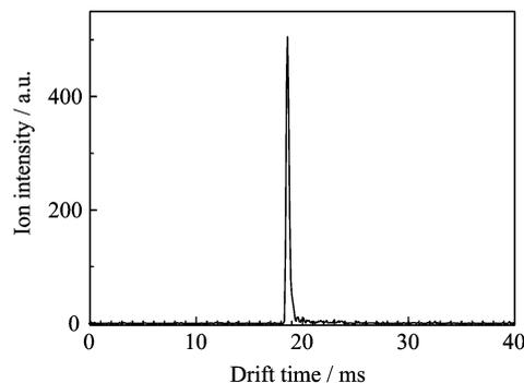
FIG. 2 High resolution ion mobility spectrum of RIP.
