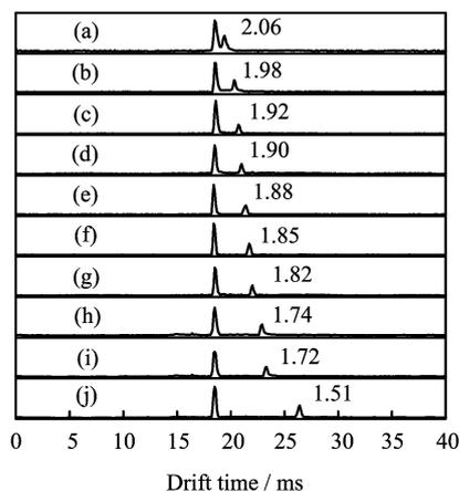
FIG. 3 Ion mobility spectra of ten alcohols measured in the CD-IMS. The labeled numbers beside the product ion peaks are the reduced mobilities. (a) Ethanol, (b) 2-propanol, (c) Propanol, (d) 2-methyl-2-propanol, (e) 2-butanol, (f) 2-methyl-1-propanol, (g) butanol, (h) isoamyl alcohol, (i) amyl alcohol, and (j) 2-octanol.
