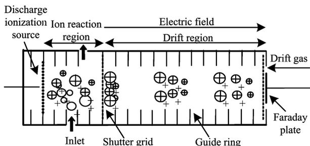
FIG. 1 Schematic diagram of ion mobility spectrometry apparatus.
