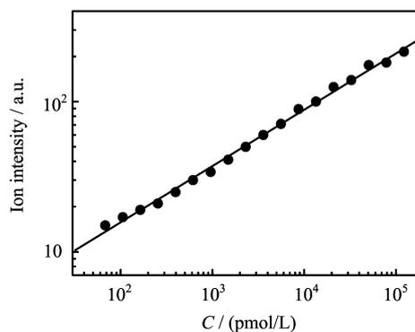
FIG. 4 Dependence of ion intensity on butanol concentration.
