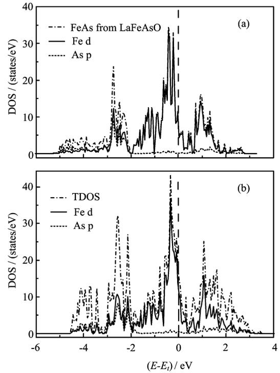
FIG. 3 Density of states of FeAs and the contributions of Fe d states and As p states to FeAs DOS. (a) PDOS of FeAs in LaFeAsO, (b) DOS of FeAs single layer with experimental values of Fe and As positions. The Fermi level is aligned to 0.00 eV.
