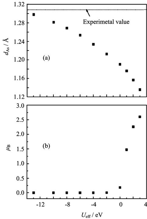
FIG. 2 Dependence of (a)  $d_{As}$  and (b) magnetic moment ( $\mu_B$ , magnetic moment of  $0.48\mu_B$  per Fe atom) on Hubbard parameter  $U$ . The experimental value of  $d_{As}$  for LaFeAsO is marked by a dotted line.
