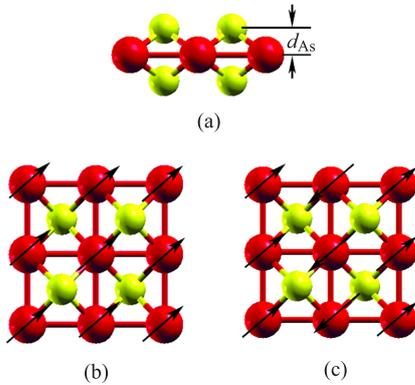
FIG. 1 The crystal structure of the  $\sqrt{2}\times\sqrt{2}\times 1$  single FeAs layer. The red and yellow balls are Fe and As species respectively. (a) The side view of single FeAs layer, (b) and (c) the top views of FeAs layer, where the black arrows signify the FM (b) and collinear AFM (c) configurations on Fe atoms. For interpretation of the color in this figure legend, the reader can refer to the web version of this article.
