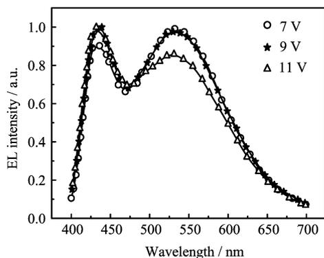
FIG. 3 EL spectra of device A at different driving voltages.
