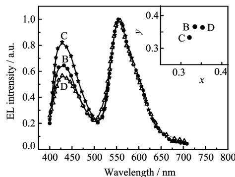
FIG. 4 EL spectra of devices with different rubrene thicknesses. Inset: Chromaticity coordinates of these devices at 7 V. B, C, and D stand for the spectra of devices with 0.1, 0.3, and 0.6 nm thick rubrene, respectively.
