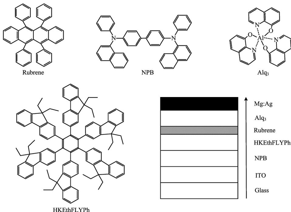
FIG. 1 Molecular structure of the used materials and device architecture.
