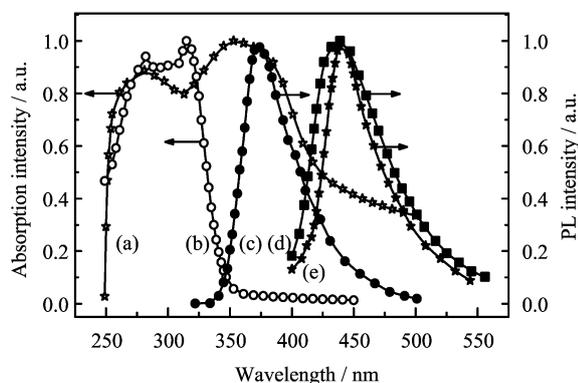
FIG. 2 Absorption and PL spectra of HKEthFLYPh and NPB films. (a) NPB absorption, (b) HKEthFLYPh absorption, (c) HKEthFLYPh emission, (d) HKEthFLYPh:NPB emission, (e) NPB emission.
