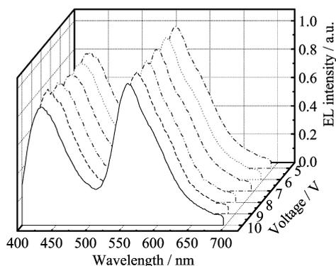
FIG. 5 EL spectra of device C biased at different applied voltages.
