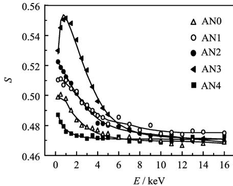
FIG. 1 Mean Doppler broadening  $S$  parameter as a function of incident positron energy  $E$  for the n-type SiC specimens AN0-AN4. The solid lines are the fitted curves.
