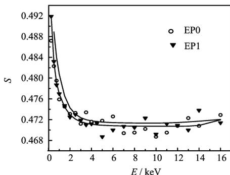
FIG. 4 Mean Doppler broadening parameter  $S$  as a function of incident position energy  $E$  for p-type SiC of specimens EP0-EP1. The solid lines are the fitted curves.
