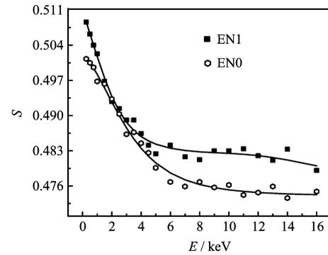
FIG. 2 Mean Doppler broadening parameter  $S$  parameter as a function of incident position energy  $E$  for n-type SiC specimens EN0-EN1. The solid lines are the fitted curves.
