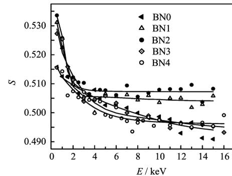
FIG. 3 Mean Doppler broadening parameter  $S$  parameter as a function of incident positron energy  $E$  for n-type electron-irradiated specimens of the second group. The solid lines are the fitted curves.
