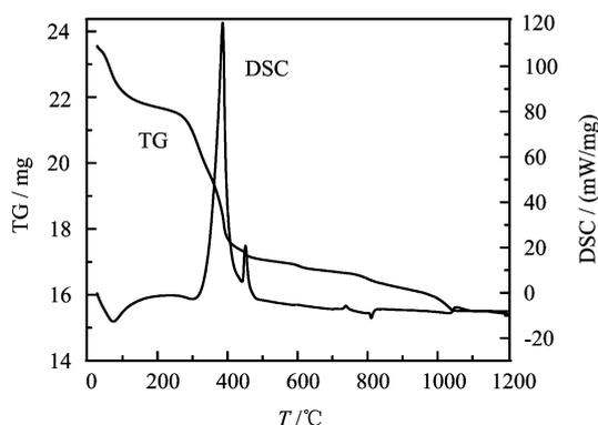
FIG. 1 DSC/TG curves of the BaTiO<sub>3</sub> nanocrystal precursor.
