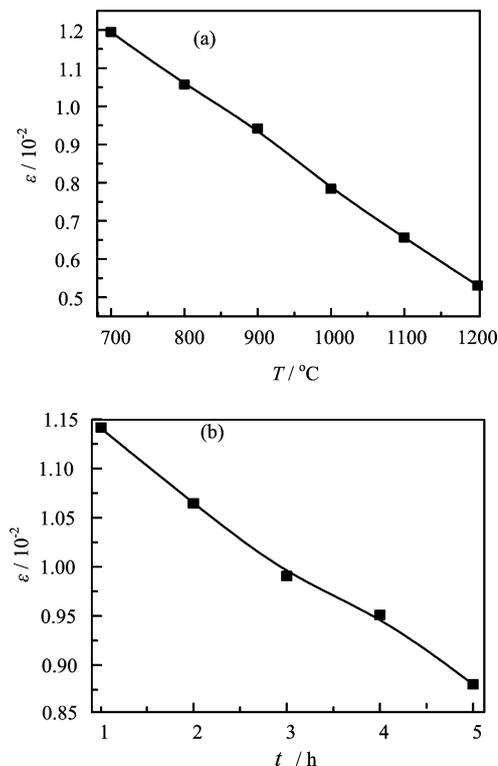
FIG. 4 (a) Effect of calcination temperature on the lattice distortion degree of BaTiO<sub>3</sub> nanocrystals calcined for 2 h and (b) effect of calcination duration on the lattice distortion degree of BaTiO<sub>3</sub> nanocrystals calcined at 800 °C.
