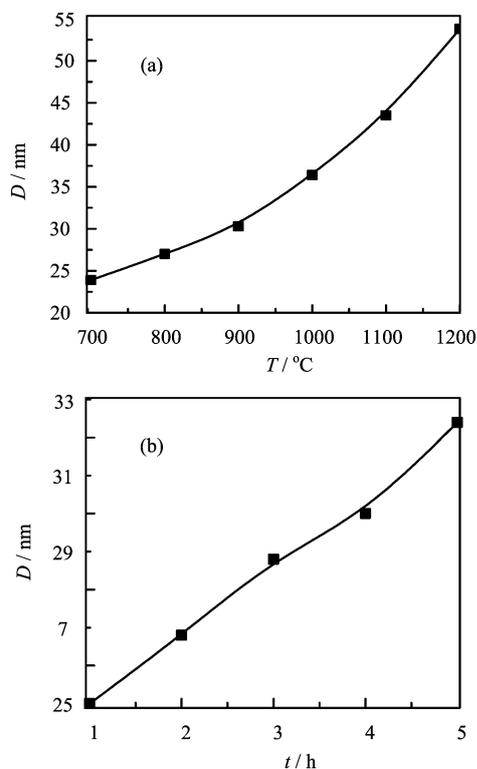
FIG. 5 Variation of grain size of BaTiO<sub>3</sub> nanocrystal with calcination temperature and calcination duration. (a) BaTiO<sub>3</sub> nanocrystal was calcined at different temperatures for 2 h. (b) BaTiO<sub>3</sub> nanocrystal was calcined at 800 °C for different durations.
