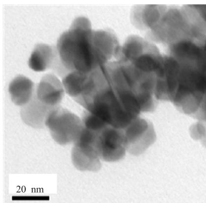
FIG. 3 TEM images of BaTiO<sub>3</sub> nanocrystals calcined at 1000 °C for 2 h.
