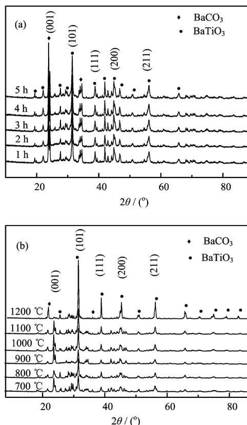
FIG. 2 XRD patterns of BaTiO<sub>3</sub> nanocrystals (a) calcined at 800 °C for different durations and (b) calcined at different temperatures for 2 h.
