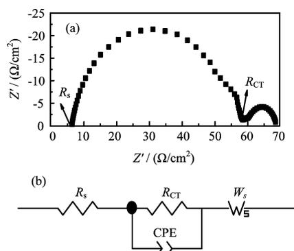
FIG. 1 (a) A typical impedance spectrum of liquid electrolyte; (b) Equivalent circuit for the impedance spectrum.  $R_s$ : Ohmic serial resistance.  $R_{CT}$ : Charge transfer resistance.  $W_s$ : Warburg impedance. CPE: Constant phase element.
