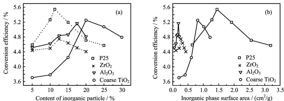
FIG. 4 Photo-electric conversion efficiency of the DSCs as a function of (a) oxide content and (b) oxide surface area.
