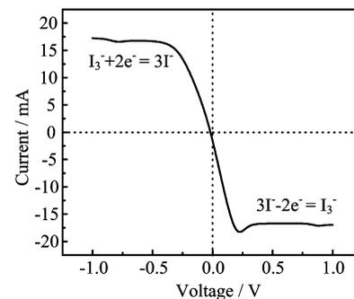
FIG. 3 Cyclic voltammogram of a typical liquid electrolyte with P25 added.
