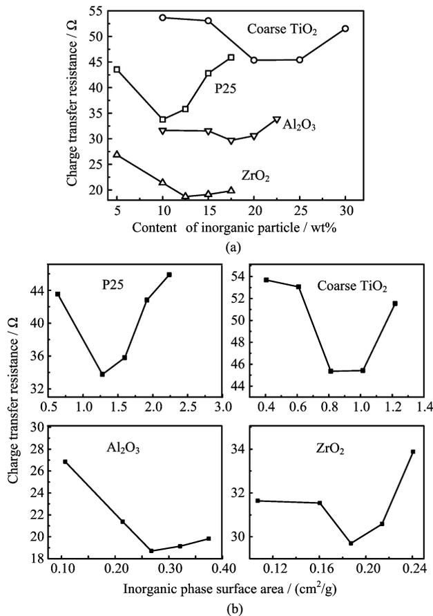
FIG. 2 Charge transfer resistance as a function of inorganic oxide particle content, and inorganic oxide particle surface area.
