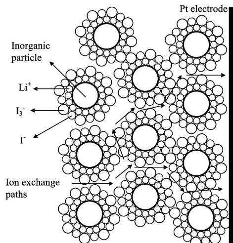
FIG. 5 Schematic diagram of ion conduction in liquid/inorganic-particle electrolyte.
