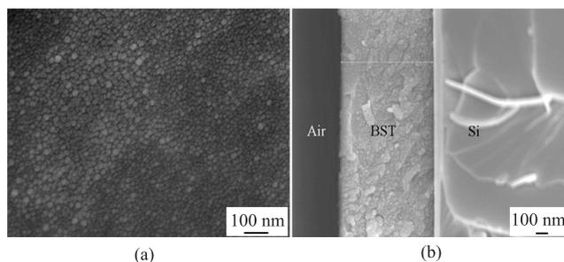
FIG. 2 FESEM photographs of BST thin films deposited at 600 °C and annealed at 700 °C. (a) The surface photograph, (b) The cross-sectional photograph.
