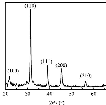
FIG. 1 The XRD patterns of BST thin films deposited at 600 °C and subsequently annealed at 700 °C.
