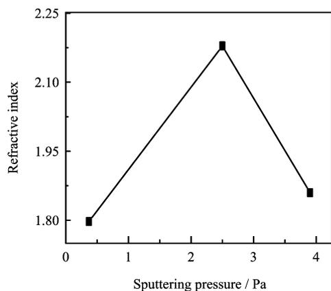
FIG. 5 The curve of refractive index of as-deposited thin films vs. pressure (at  $\lambda=550$  nm).
