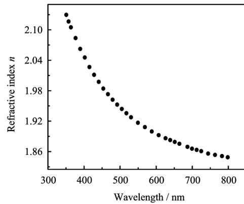
FIG. 4 Refractive index of  $Ba_{0.65}Sr_{0.35}TiO_3$  thin films as a function of wavelength.
