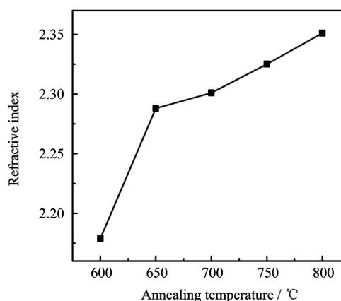
FIG. 6 Refractive index curve of  $\text{Ba}_{0.65}\text{Sr}_{0.35}\text{TiO}_3$  thin films for as-deposited and post-deposited annealed at 650, 700, 750, and 800 °C (at  $\lambda=550$  nm).
