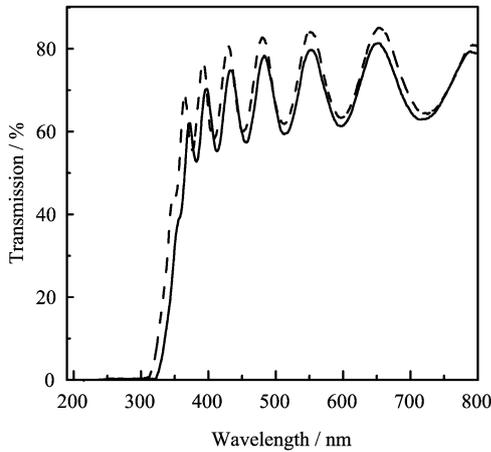
FIG. 3 Optical transmittance spectra of BST thin films deposited on fused quartz substrates: (a) 700 °C (---); (b) 800 °C (—).
