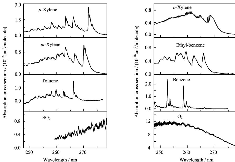
FIG. 4 The absorption cross sections of BTX [5].
