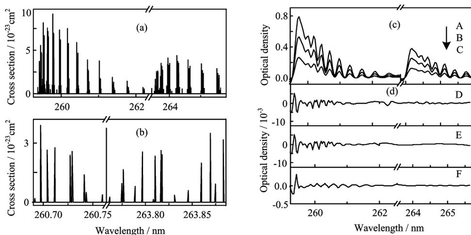
FIG. 8 The 4-0 and 5-0 vibronic band of the Herzberg I band system of O<sub>2</sub> [23]. (a) High resolution absorption cross section. (b) Two part of cross section shown in layer (a). (c) The shown spectra correspond to  $L=400$  m (A), 800 m (B), and 1200 m (C) ( $\Gamma=0.15$  nm). (d) The remaining residual structures (D, E, and F) after B are fitted by A and C separately and simultaneously.
