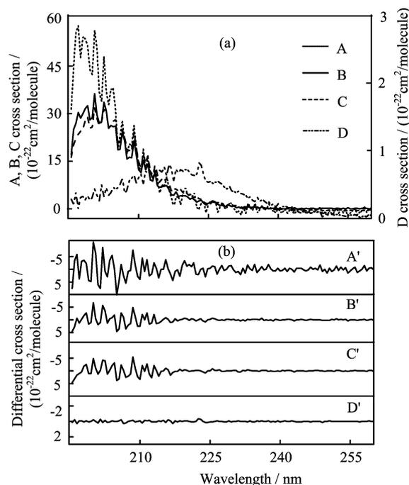
FIG. 6 The  $O_2$  absorption cross section at different temperatures and pressures. (a) A. 1073 K, 100 kPa; B. 1073 K, 400 kPa; C. 1073 K, 600 kPa; D. 293 K, 600 kPa. (b) A', B', C', and D': the resulting spectra of A, B, C, and D respectively after being high filtered.
