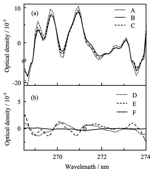
FIG. 3 The  $\text{SO}_2$  differential absorption spectra at different temperatures ( $\Gamma=0.15 \text{ nm}$ ). (a) A: 243 K, B: 273 K, C: 293 K. (b) The residual structures after fitting A to B (D), C to B (E), and A and C (simultaneously) to B (F) corresponding to optical densities of 0.9%, 0.8%, and 0.009%, respectively.
