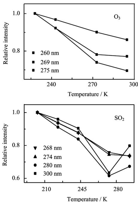
FIG. 5 The relative intensity of differential absorption spectra of  $O_3$  and  $SO_2$  at different temperatures.
