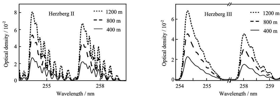
FIG. 7 Oxygen reference spectrum of the Herzberg II and III ( $\Gamma=0.15$  nm).
