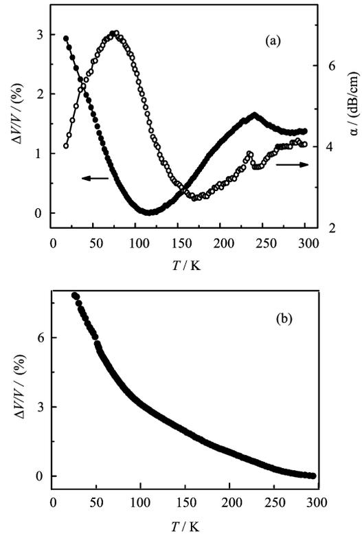
FIG. 3 (a) Temperature dependence of longitudinal ultrasonic velocity and attenuation for  $\text{La}_{1/3}\text{Sr}_{2/3}\text{CoO}_3$ . (b) The temperature dependence of the longitudinal ultrasonic velocity for  $\text{La}_{0.8}\text{Sr}_{0.2}\text{CoO}_3$ .
