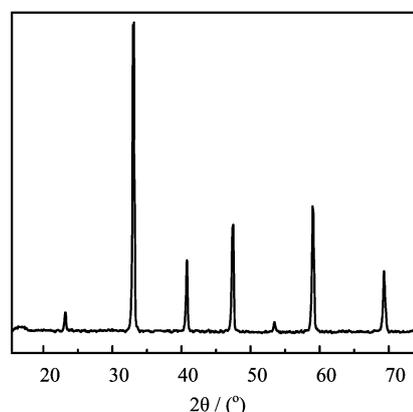
FIG. 1 XRD pattern of  $\text{La}_{1/3}\text{Sr}_{2/3}\text{CoO}_3$  at room temperature.
