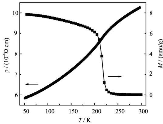
FIG. 2 Temperature dependences of resistivity and magnetization for  $\text{La}_{1/3}\text{Sr}_{2/3}\text{CoO}_3$ .
