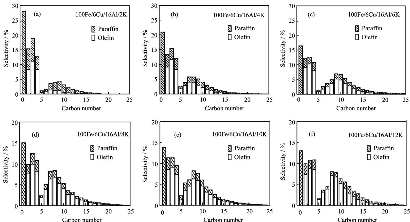
FIG. 4 The effect of potassium content on hydrocarbon products distribution over 100Fe/6Cu/16Al/ $x$ K ( $x=2-12$ ) catalysts.
