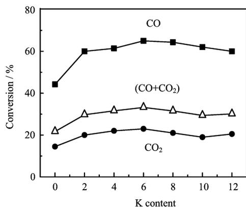
FIG. 2 Effect of potassium content on CO conversion,  $CO_2$  conversion, and total carbon ( $CO+CO_2$ ) conversion over 100Fe/6Cu/16Al/ $x$ K catalysts.
