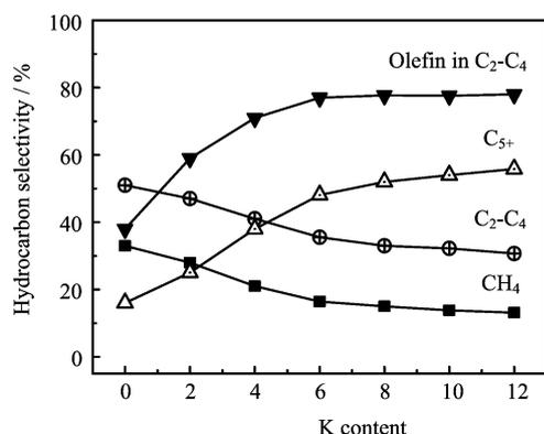
FIG. 3 Effect of potassium content on the selectivity of hydrocarbon products over 100Fe/6Cu/16Al/*x*K catalysts.
