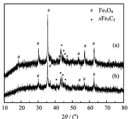
FIG. 6 XRD patterns of (a) 100Fe/6Cu/16Al/12K and (b) 100Fe/6Cu/16Al/6K after activity test of 80 h.
