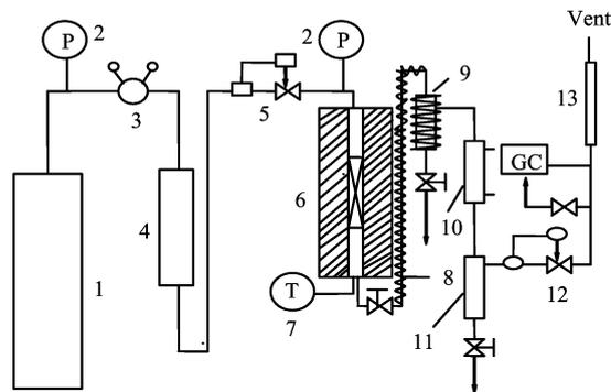
FIG. 1 Schematic diagram of experimental apparatus for Fischer-Tropsch synthesis using the bio-oil-syngas. 1. Bio-oil-syngas, 2. Pressure gauge, 3. Pressure regulator (YT-2), 4. Gas purifier, 5. Mass flow controller, 6. Fixed bed reactor, 7. Thermocouple, 8. Electric heating strip, 9. Wax collector, 10. Water-cool vessel, 11. Liquid product condenser, 12. Back pressure regulator, 13. Soap flowmeter.
