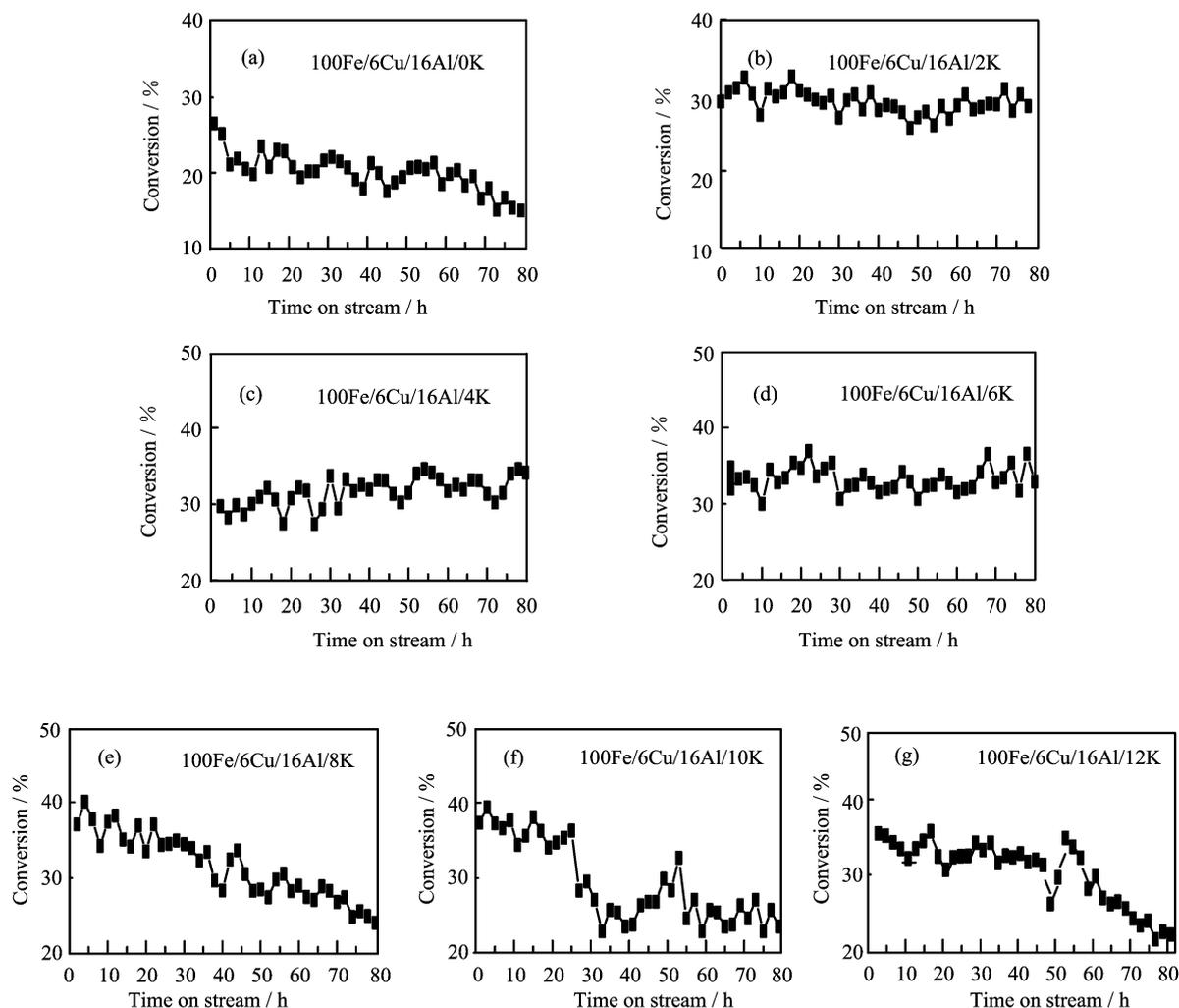
FIG. 5 Effect of time on stream on the total carbon ( $\text{CO}+\text{CO}_2$ ) conversion using  $100\text{Fe}/6\text{Cu}/16\text{Al}/x\text{K}$  ( $x=0-12$ ) catalysts with different K content.
