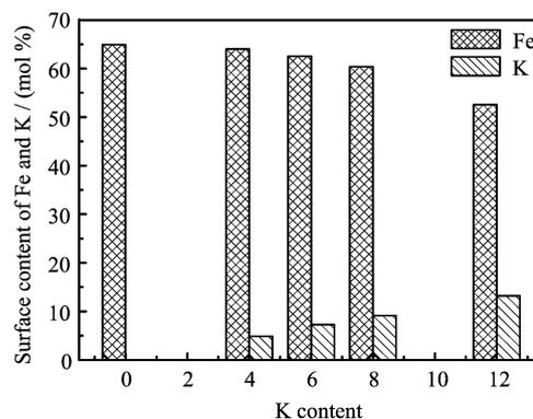
FIG. 7 The effect of potassium content (*x* value, *x*=0, 4, 6, 8, 12) on the surface content (mol%) of Fe and K.
