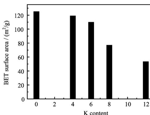
FIG. 8 The effect of potassium content on the BET surface area of the 100Fe/6Cu/16Al/*x*K (*x*=0, 4, 6, 8, 12).
