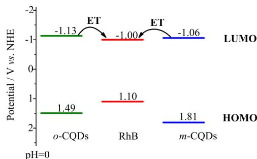
FIG. 3 The energy-level diagram for the three bare samples of *o*-CQDs, RhB, and *m*-CQDs.
