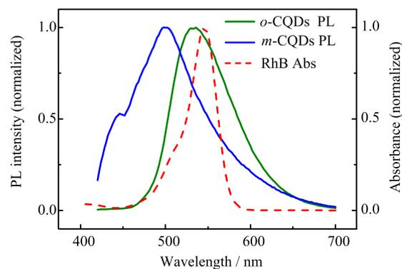
FIG. 1 The normalized steady-state PL spectra of *o*-CQDs and *m*-CQDs (solid lines) as well as the normalized steady-state UV-Vis absorption spectrum of RhB (dashed line).
