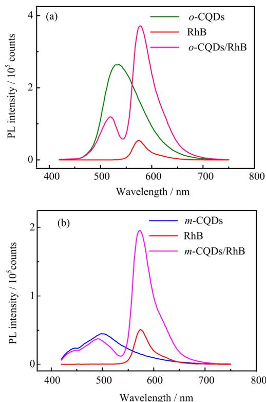
FIG. 2 The steady-state PL spectra of (a) *o*-CQDs, RhB, and *o*-CQDs/RhB and (b) *m*-CQDs, RhB, and *m*-CQDs/RhB.
