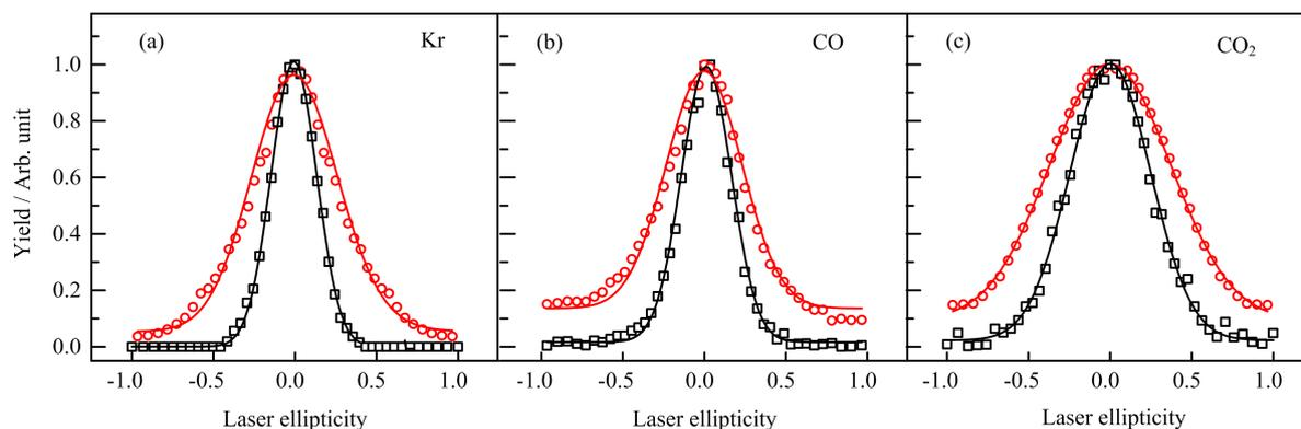
FIG. 4 The yield of double ionization as a function of laser ellipticity for (a) Kr, (b) CO, and (c) CO<sub>2</sub> at  $1 \times 10^{14}$  W/cm<sup>2</sup> (black square) and  $2 \times 10^{14}$  W/cm<sup>2</sup> (red circle). The solid curves show the best-fit Gaussian distributions to the experimental data.
