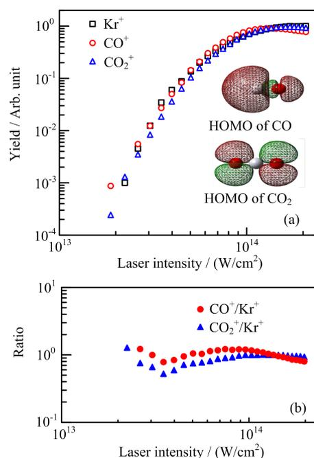
FIG. 2 (a) The single ionization yields of Kr (black hollow square), CO (red hollow circle) and CO<sub>2</sub> (blue hollow triangle) as a function of laser intensity. The HOMOs of the molecules are also shown. (b) The ratio between molecule and atom are shown for CO (red solid circle) and CO<sub>2</sub> (blue solid triangle) at different laser intensities.
