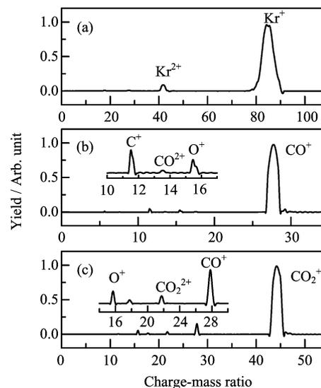
FIG. 1 Time-of-flight mass spectra of (a) Kr, (b) CO, and (c)  $CO_2$  at  $1 \times 10^{14}$  W/cm<sup>2</sup>.
