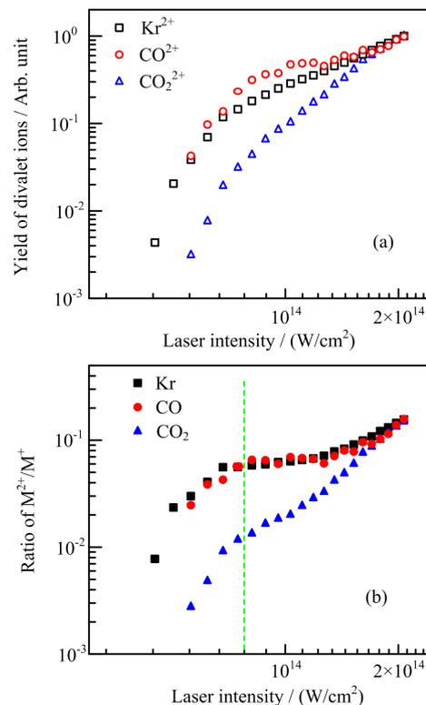
FIG. 3 (a) The double ionization yields of Kr (black hollow square), CO (red hollow circle) and CO<sub>2</sub> (blue hollow triangle) as a function of laser intensity. All the three curves are normalized to its maximum respectively. (b) The laser intensity dependence of M<sup>2+</sup>/M<sup>+</sup> for Kr (black solid square), CO (red solid circle) and CO<sub>2</sub> (blue solid triangle). The green line indicates the “knee” structure at  $8 \times 10^{13}$  W/cm<sup>2</sup>.
